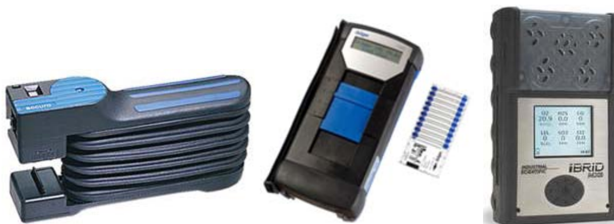
Figure 11: Gas monitoring devices: Draeger Tube Bellows {left}, Draeger CMS with ten chemical specific chips {center}, iBRID MX6 multi-gas monitor {right}
