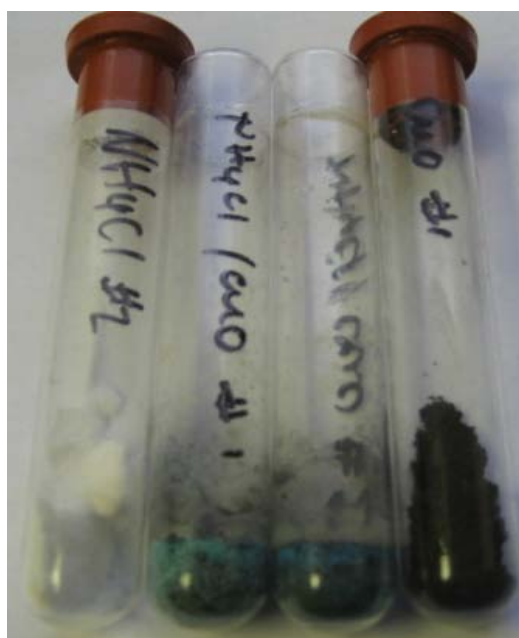
Figure 23: “Aged” VTS tubes containing NH 4 Cl {left}; 2-tubes of NH 4 Cl/Cupric Oxide {center}; Cupric Oxide {right}
