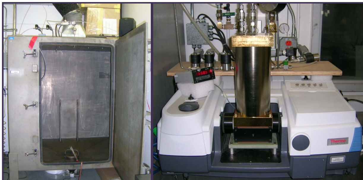
Figure 12: Autoliv test equipment: 100 cubic foot chamber {left}, FT-IR {right}
