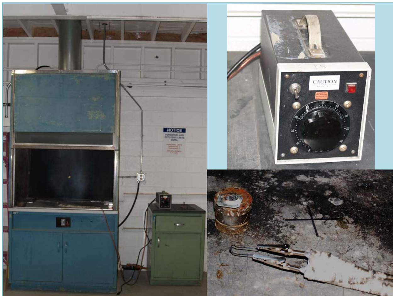
Figure 7: Test equipment used for initial obscurant formulation screening. Hood designated for ignition and combustion characterization of 0.05-5.0 grams of pyrotechnics {left}, variable output power supply {top right}, sample holder and ignition wand with tungsten ignition wire {bottom right}
