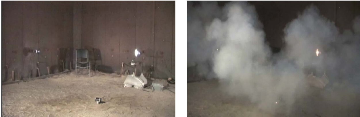
Figure 17: Test setup {left} and smoke output {right} of an IFBG containing an 18.2-gram net explosive weight shown two seconds after initiation of the grenade.
