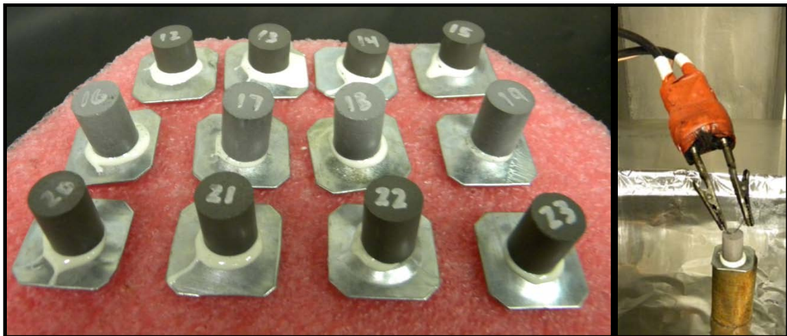
Figure 9: HCE obscurant replacement samples prepared for testing {left}, pellet ready for ignition {right}
