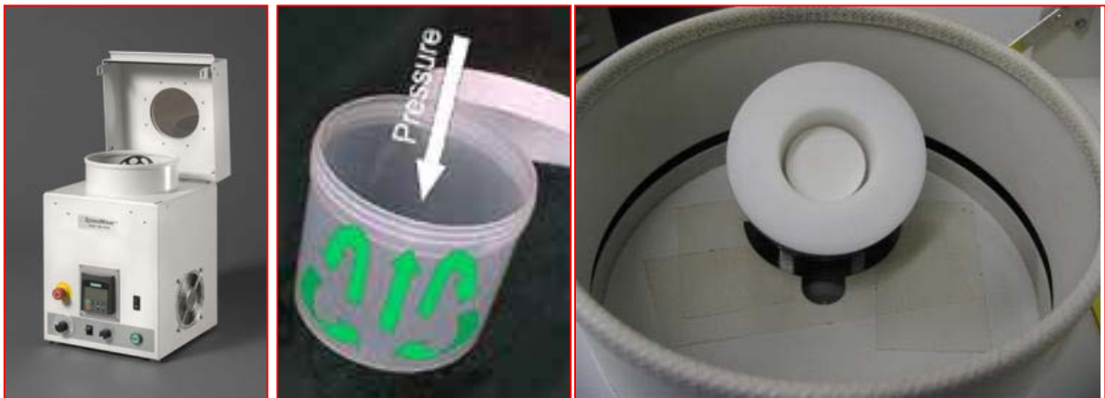
Figure 1: FlackTek SpeedMixer {left}, mixing cup {center}, SpeedMixer mixing compartment with mixing cup placed cup holder system {right}
