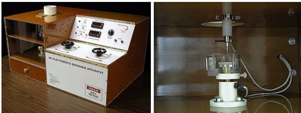
Figure 4: ABL ESD test apparatus {12}, close-up view of the ESD needle, stand and sample enclosure {right}
