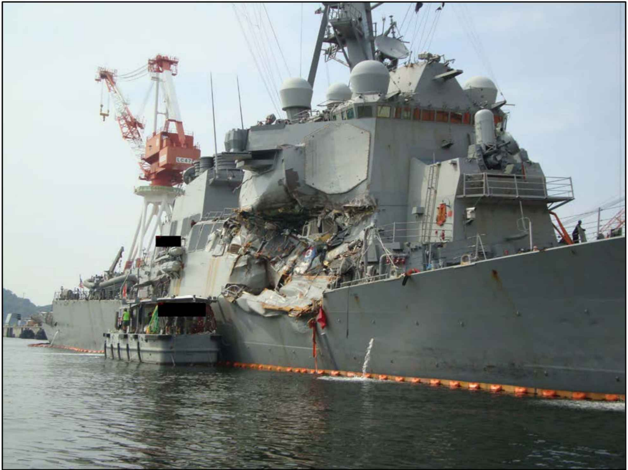
Figure 8. Post collision damage to the Fitzgerald 's starboard side. (Source: US Navy)
