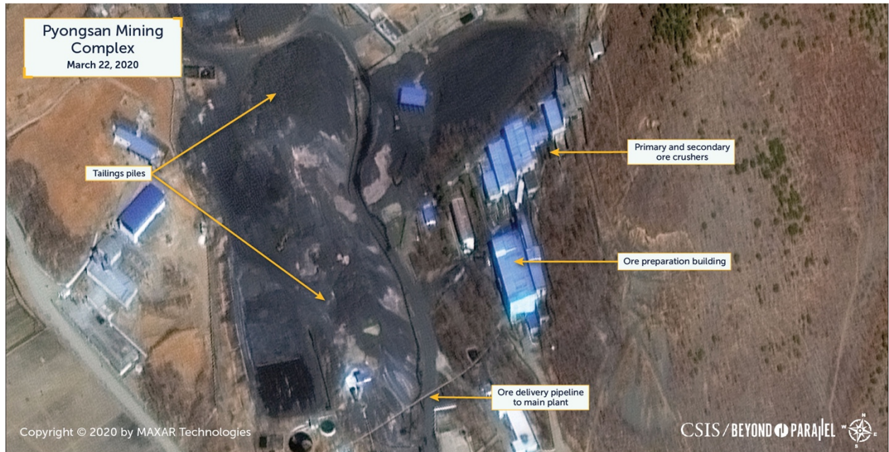
Overview of the Pyongsan Uranium mining complex located northeast of the main plant as of March 22, 2020. (Copyright © 2020 by Maxar Technologies)
