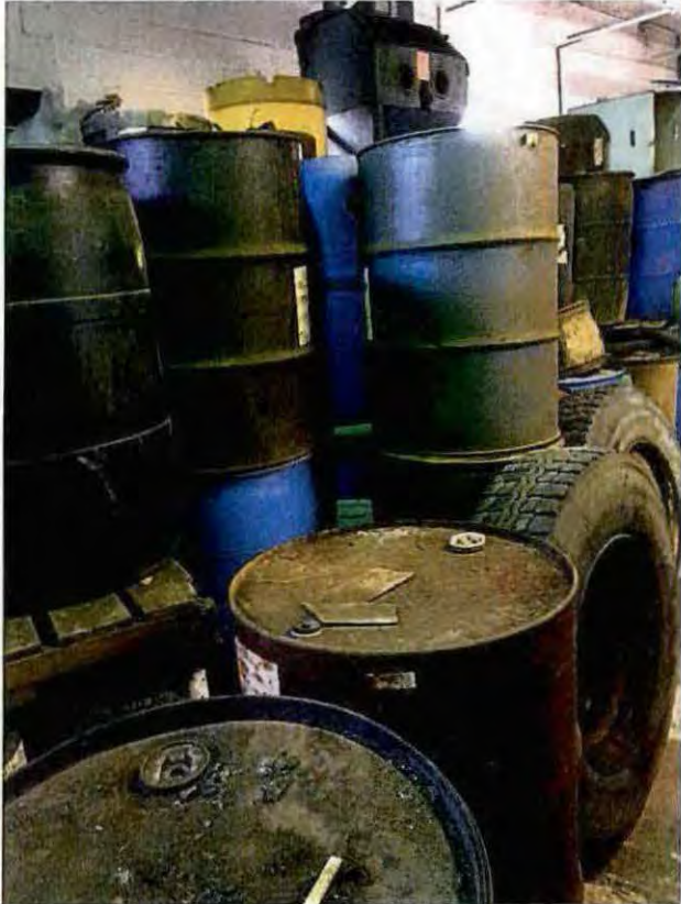
Photo 45: Representative container storage in adjacent building, some unlabeled and compatibility with acid unknown
