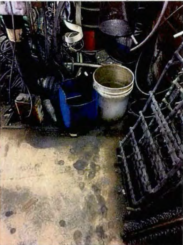
Photo 32: Purported containers of Trichloroethylene for degreasing on plating bath floor
