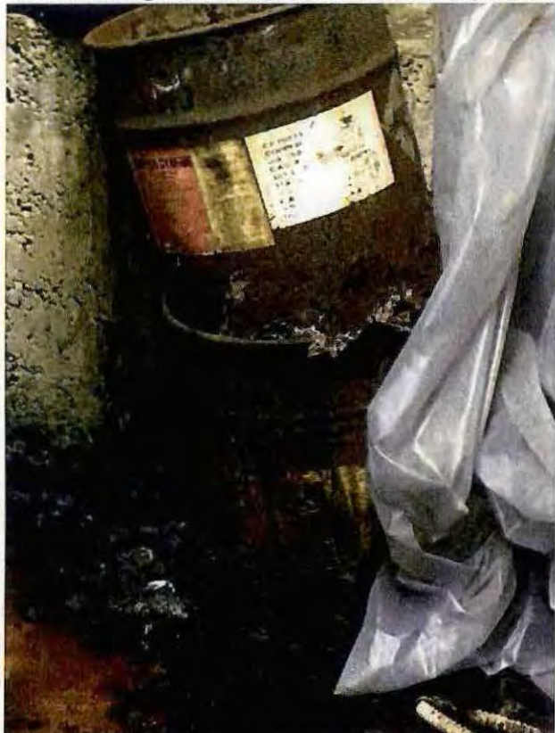
Photo 21: Corroded and leaking containers with "Copper Cyanide" label in basement
