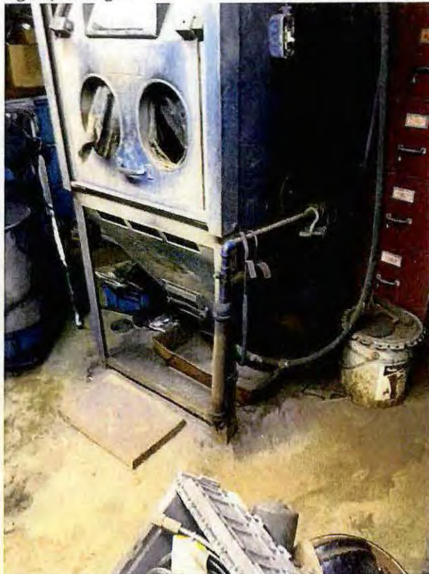
Photo 10: "Sand blast cabinet" – aluminum oxide shavings
