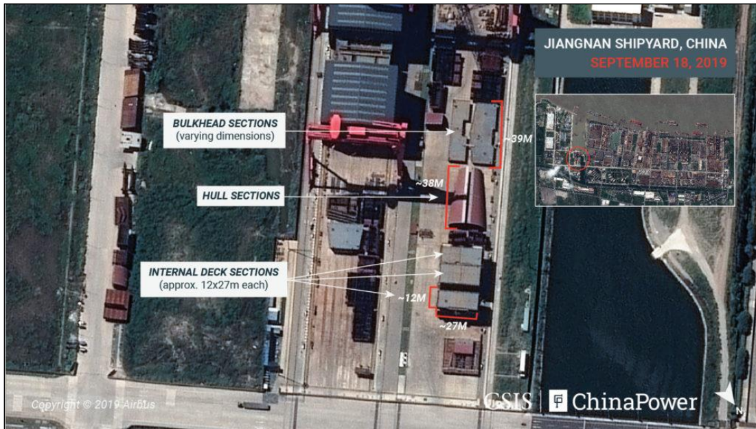
Figure 9. Type 002 Aircraft Carrier Under Construction
