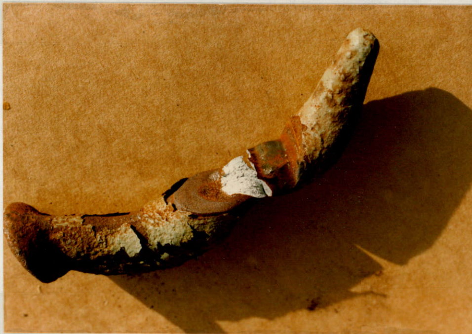
Figure 4. This hook shows the point of failure to be in the worn section of the bowl-saddle.
