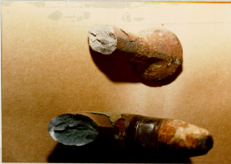
Figure 5. This hook failed at the heel even though it had approximately the same wear pattern in the bowl-saddle as the hook in Figure 4.
