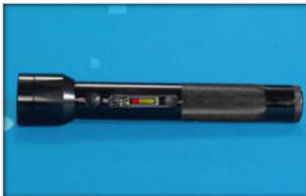
Figure 2. PAS III, a standard police flashlight with a built-in passive alcohol sensor
