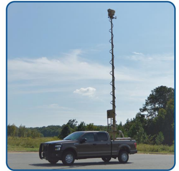
Mobile Video Surveillance System (MVSS)
