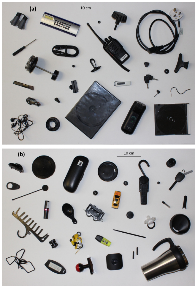
Fig. 1. Examples of EEE and non-EEE samples that were Pb-positive (a) and non-EEE samples that were Br-positive (b).
