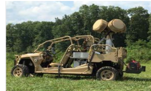
Figure 1. L-MADIS w/MODi RF jammer and RPS-42 sensor
