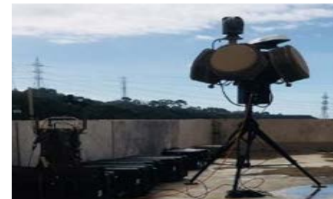
Figure 3. E-MADIS with RPS-42 and MODi on a rooftop
