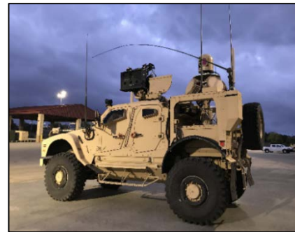
Inc 1 MADIS Mk2 (Sensor, C-UAS interceptor, gun, EW)
