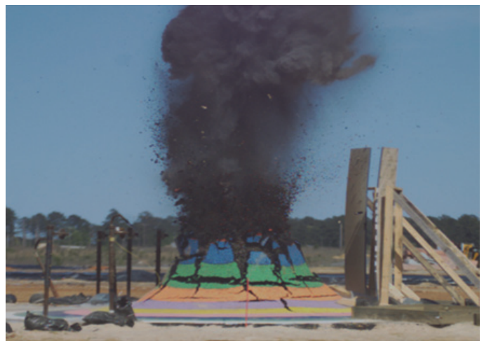
Figure 2. Buried Ordnance Test using a simulated asphalt roadbed. Results from such tests are used to choose strike packages that achieve desired effects while minimizing collateral damage.
