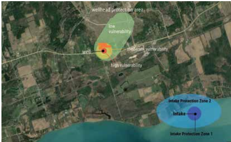
Figure 2. Vulnerable areas that require special protection from drinking water threats. Generally, the areas closest to a wellhead or surface water intake are considered most vulnerable.
