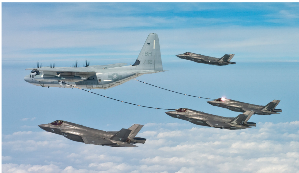
Figure 10: F-35B Aircraft Refuel from a KC-130 Aerial Refueling Tanker Using Hose and Drogue Refueling Equipment
