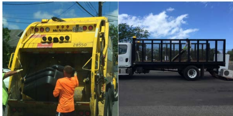
Exhibit 2.2 Rear Loading Packer Truck (left) and Flatbed Truck (right)
