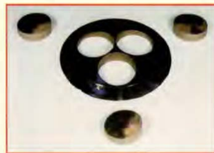
A shallow, 2-cm-diameter metal sample provides three miniature test specimens.
