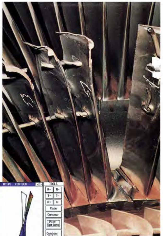
BLADE FAILURE A leading cause of steam turbine unavailability is blade failure, which can follow rapidly after the first appearance of cracking. To predict when such cracking will begin, the BLADE computer program calculates the vibration characteristics and local strain responses of a given group of turbine blades.
