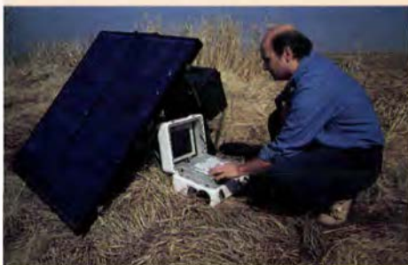
The Automated Wildlife Surveyor (AWS), shown here with an optional photovoltaic system, uses microphone technology to monitor wildlife.
