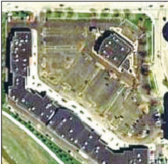
Parking lot redesign. The original design to the left used conventional straight parking bays, poorly adapted to the building configuration. The result was numerous conflicts, disorienting angles, and awkward intersections. The parking lot redesign at right used curved parking bays to provide 90-degree intersections and eliminated most multi-point intersections, while adding parking stalls through more-efficient circulation.
