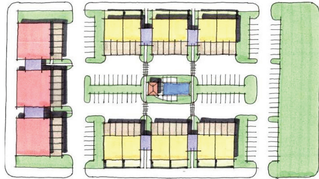
Diagram of a multifamily project with interior parking and buildings along the street frontages. Garages are incorporated into the rear facades of buildings.
