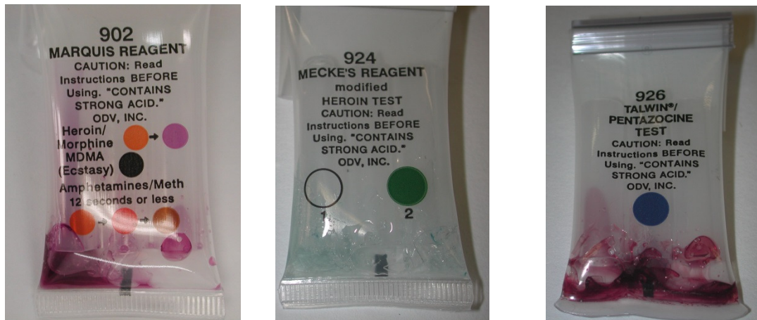
Figure 5: Color results of white heroin: Marquis – purple, Mecke – bluish/green, and Froehde – purple using NarcoPouches
