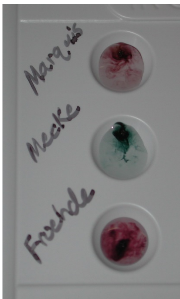
Figure 6: Color results of black tar heroin: Marquis – purple, Mecke – bluish/green and Froehde – purple using laboratory prepared chemicals
