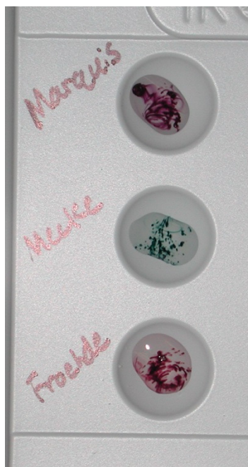
Figure 4: Color results of white heroin: Marquis – purple, Mecke – bluish/green, and Froehde – purple using laboratory prepared chemicals
