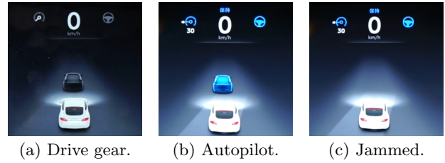
Figure 9: Tesla dashboard display at drive gear, Autopilot, and Autopilot under radar jamming.
