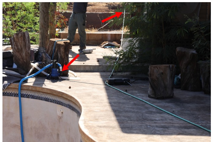
Figure 4.3.5.3.11 Water resources from 1█ Kaniau Road were utilized to help control the fire from propagating farther east (mauka) from 1█ Kaniau Road. Garden hose was deployed from a hose bib with the terminal end remaining at the next lot. Neighbors reportedly used the pump to control a fire along the plastic fence at the north property line of this lot.
