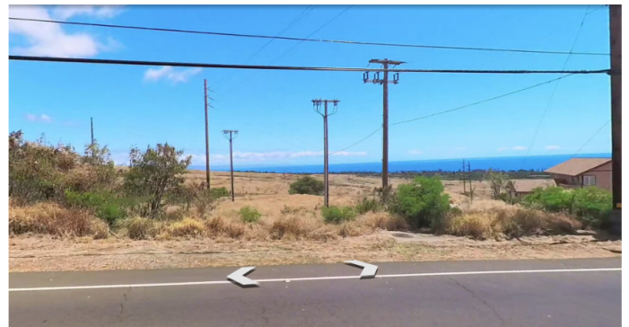
Figure 3.7.7.5 Google Street View image (pre-fire, date unknown) looking south from Lahainaluna Road. Home in the image is addressed at 8█ Ho'okahua Street and was the structure nearest the Lahaina AM fire point of origin. Image shows buffelgrass and haole koa at the base of several utility poles supporting overhead electrical lines. Inset: Viewpoint of the image above.
