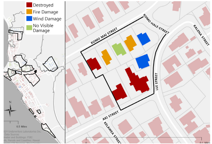
Figure 4.3.3.2 Damage classification assessment map of Kahoma subdivision analysis area.
