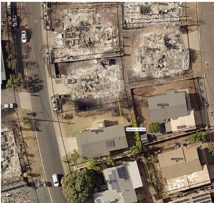
Figure 4.3.5.2.11 (Left) Post-fire aerial image with annotated distance, 39 feet, between (destroyed) 12█ 'Ainakea Road and (damaged) 12█ 'Ainakea Road. (Right) Ground-based image of separation between destroyed and damaged structures.
