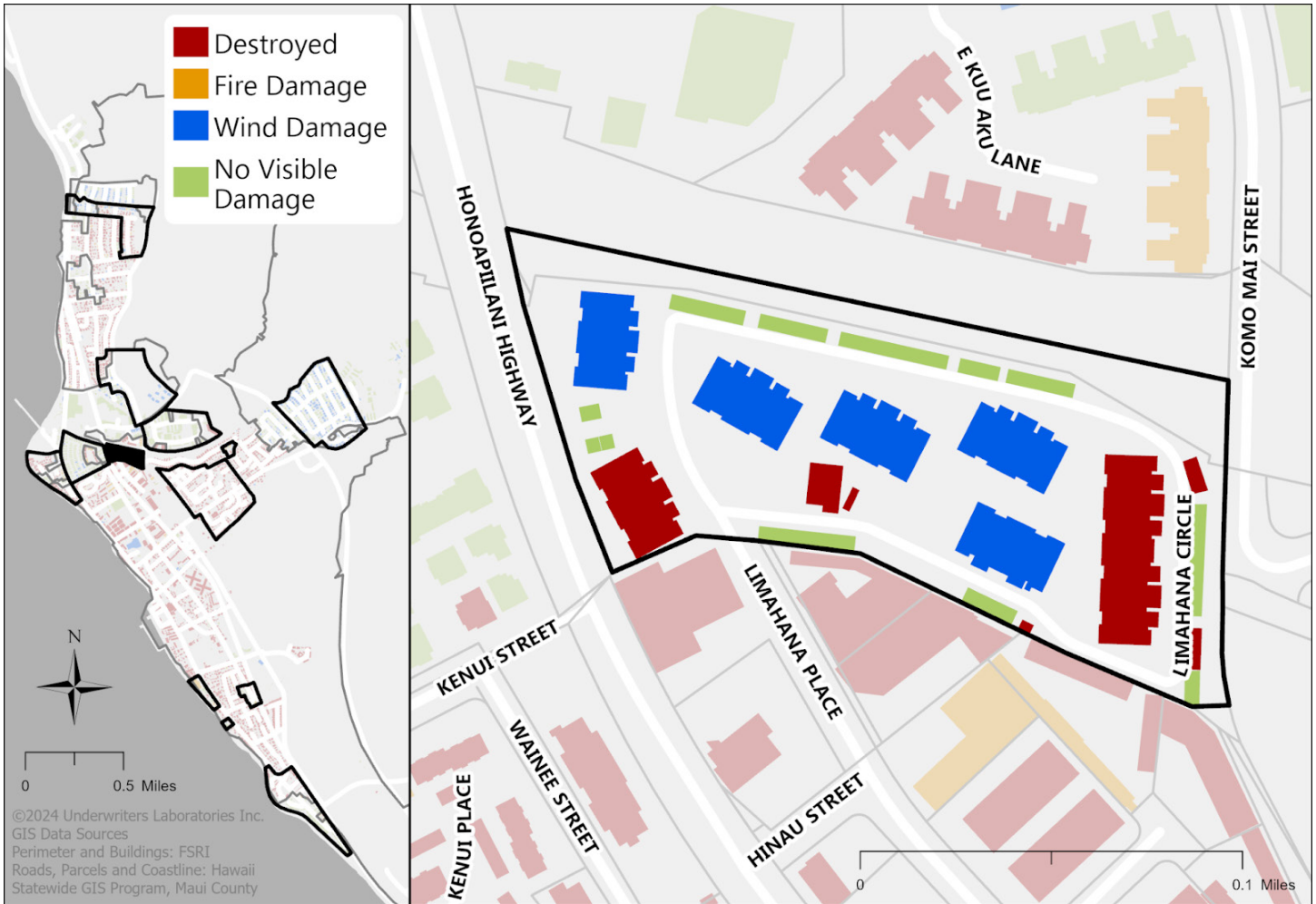
Figure 4.3.3.4.2 Damage classification assessment map of Opukea apartment complex analysis area.
