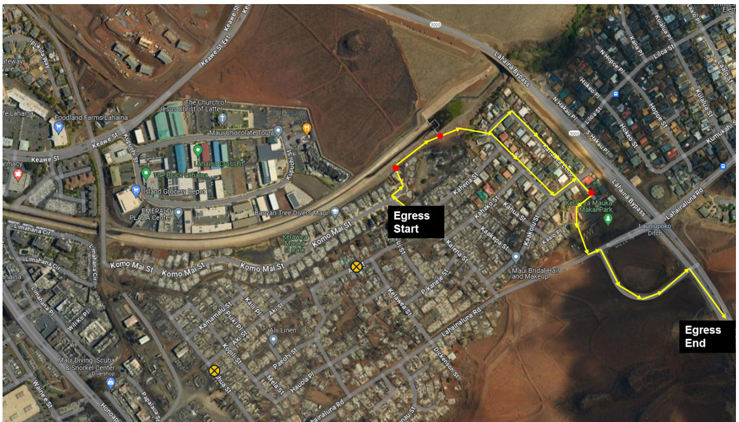
Figure 4.3.3.1.7 Map showing egress route at 16:41 after the fire cut off the westbound exits via Komo Mai Street and Lahainaluna Road. Orange dots represent the location of the fallen trees and debris blocking Kuhua and Aki Streets. Red dots represent locked gates that police officers and residents forcibly opened to gain access to alternative egress routes depicted by the yellow lines.
