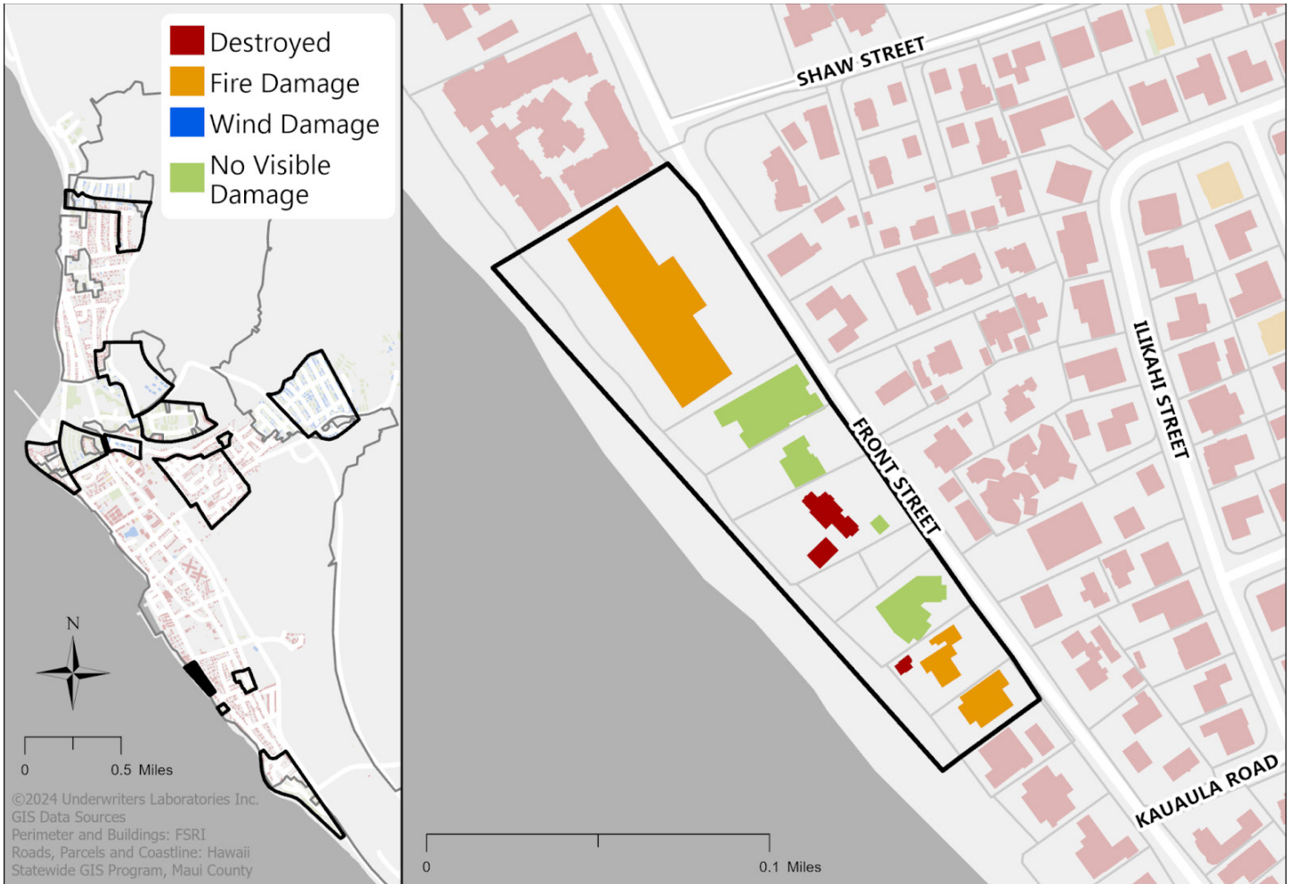
Figure 4.3.4.1.2 Damage classification assessment map of the 400 block of Front Street analysis area.
