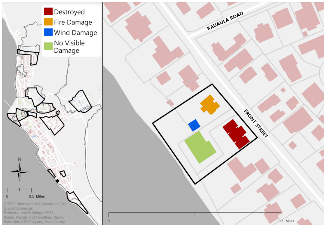
Figure 4.3.4.3.2 Damage classification assessment map of analysis area.
