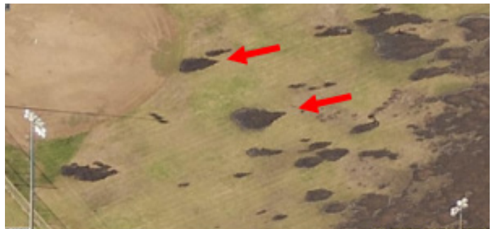
Figure 4.3.4.1.3 The orientation of wind impacting the 400 block of Front Street in Lahaina can be visualized in the grass fields on either side of Mill Street, around the Lahaina Aquatic Center and Boys & Girls Clubs of Maui (middle). Representative damage to trees oriented towards the west (makai) (bottom). Spot fire damage in the softball field, where the heel of the fire can be identified towards the east (mauka), indicating spread to the west (makai)—assuming flat terrain on the grass field (top).
