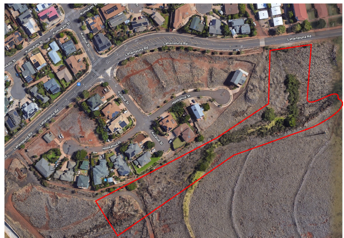
Figure 3.7.7.2 Google Earth pre-fire image (July 9, 2016) of the area where the Lahaina AM fire burned. Red outline marks the ravine with walls made of large boulders that contained voids where tufts of dry vegetation and combustible trash were concealed. The area outlined is approximately five (5) acres.
