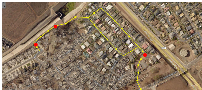
Figure 3.8.2.4 Evacuation route used by residents exiting the Lahainaluna neighborhood as the fire burned through the Lahainaluna neighborhood. Route required breaking open three (3) locked gates (red circles), and driving on dirt roads to make access to Lahainaluna Road, and ultimately, the Lahaina Bypass.
