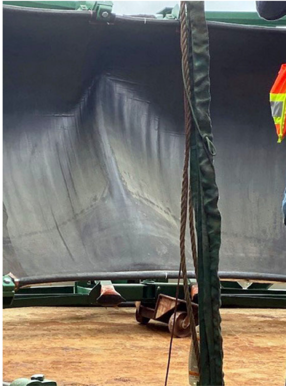
Figure 10: Damaged Rubber Window of Sonar Dome
