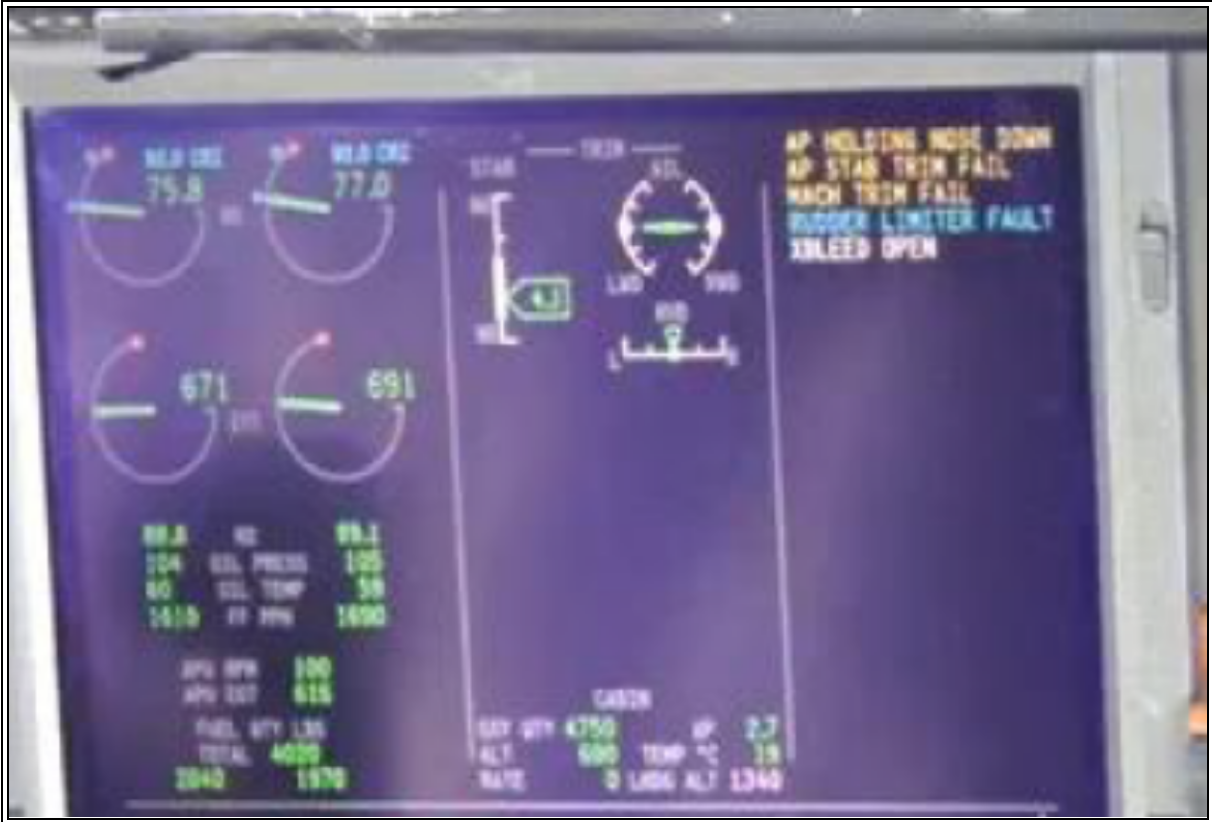
Figure 8: View of the flight test vehicle in-flight with the CAS displaying a series of caution messages and advisory messages.
