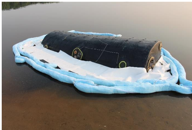
Photo 2 - Right side fuel cell (with POL absorbent material)
