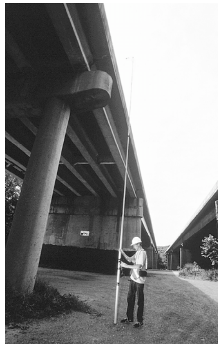
Figure 18. To survey unreachable roosts, researchers use a camera lens attached to a telescoping pole.
