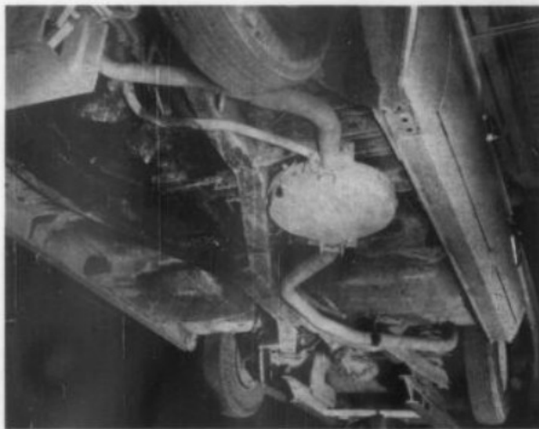
EXHAUST-CONTROL DEVICES are now in the mill which would reduce hydrocarbon and CO emissions considerably. Pictured is the catalytic converter developed jointly by Universal Oil Products Co. and Oxy-Catalyst, Inc.
