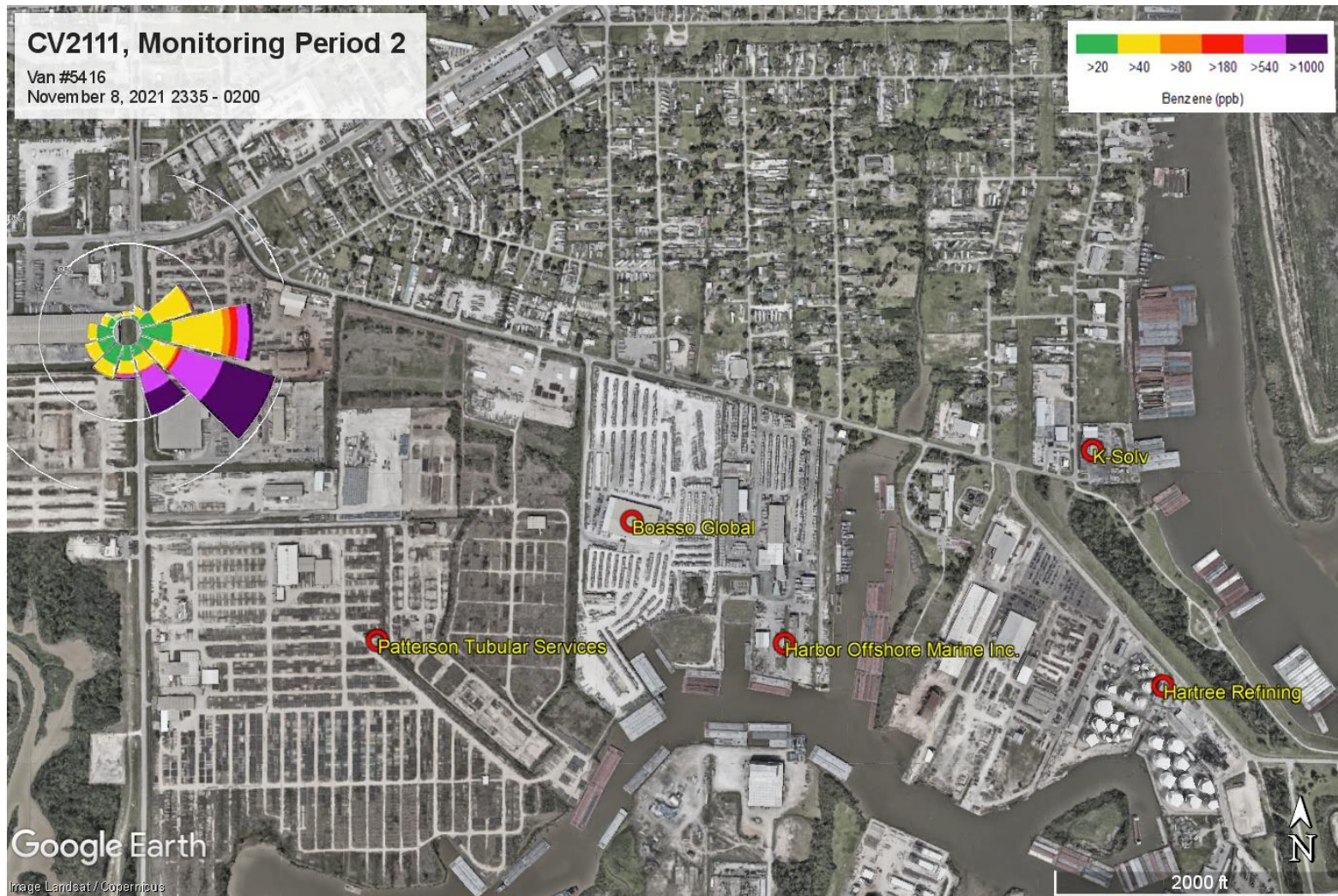
Figure 4: Van #5416 11/8/2021 ST10 stationary monitoring location with maximum instantaneous benzene concentration of 2487.9 ppbv and maximum 1-hour benzene average concentration of 534.6 ppbv on Sheldon Rd approximately 0.1 miles south of Market St in Channelview, Texas (29.770354, -95.12444). This map was generated by the Monitoring Division of the Texas Commission on Environmental Quality. This product is for informational purposes and may not have been prepared for or be suitable for legal, engineering, or surveying purposes. It does not represent an on-the-ground survey and represents only the approximate relative location of property boundaries. For more information concerning this map, contact the Monitoring Division at 512-239-1716.
