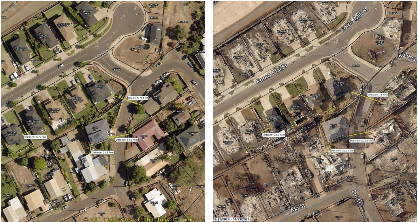
Figure 4.3.3.3.1 Pre- and post-fire aerial imagery of homes that survived the fire on Komo Mai Street and Lu'i Street. Annotations depict separation distances between perimeter structures and nearest destroyed structure.
