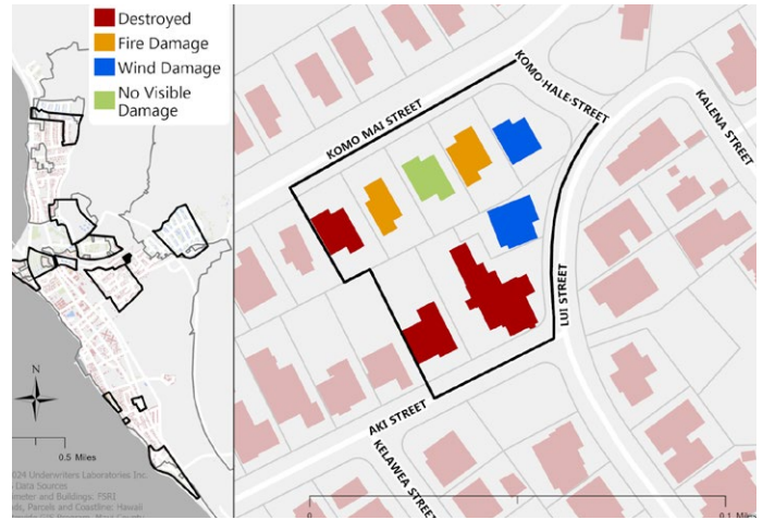
Figure 4.3.3.3.2 Damage classification assessment map of Kahoma subdivision analysis area.
