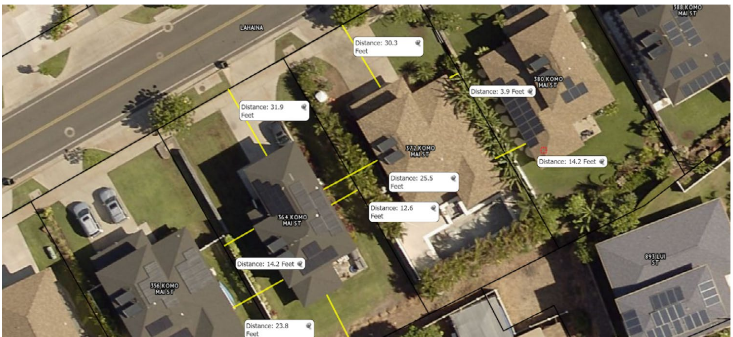
Figure 4.1.3.1 Example of distance measurement capabilities with aerial imagery and potential reference point for set back and separation distances.
