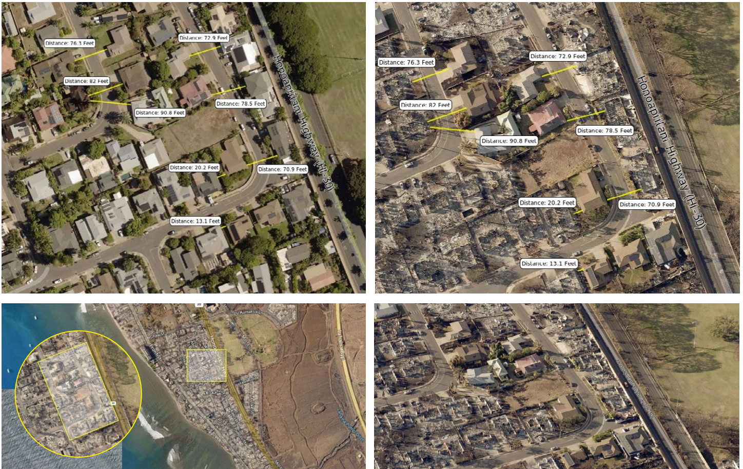
Figure 4.3.4.2.3 Surviving cluster of structures along the 400 block of 'Āli'ō Street and Waine'e Street including east (mauka)-west (makai) separation distances on (top right) pre-fire image and (bottom right) post-fire image. Inset: Viewpoint showing area depicted in photographs above.
