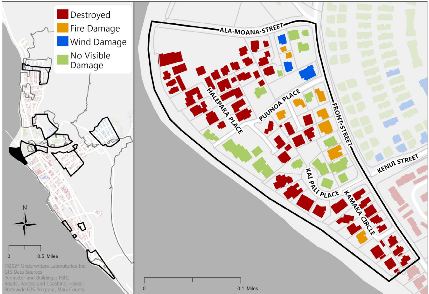
Figure 4.3.3.6.2 Damage classification assessment map of Front Street to the beach between Ala Moana Street and Kamaka Circle analysis area.
