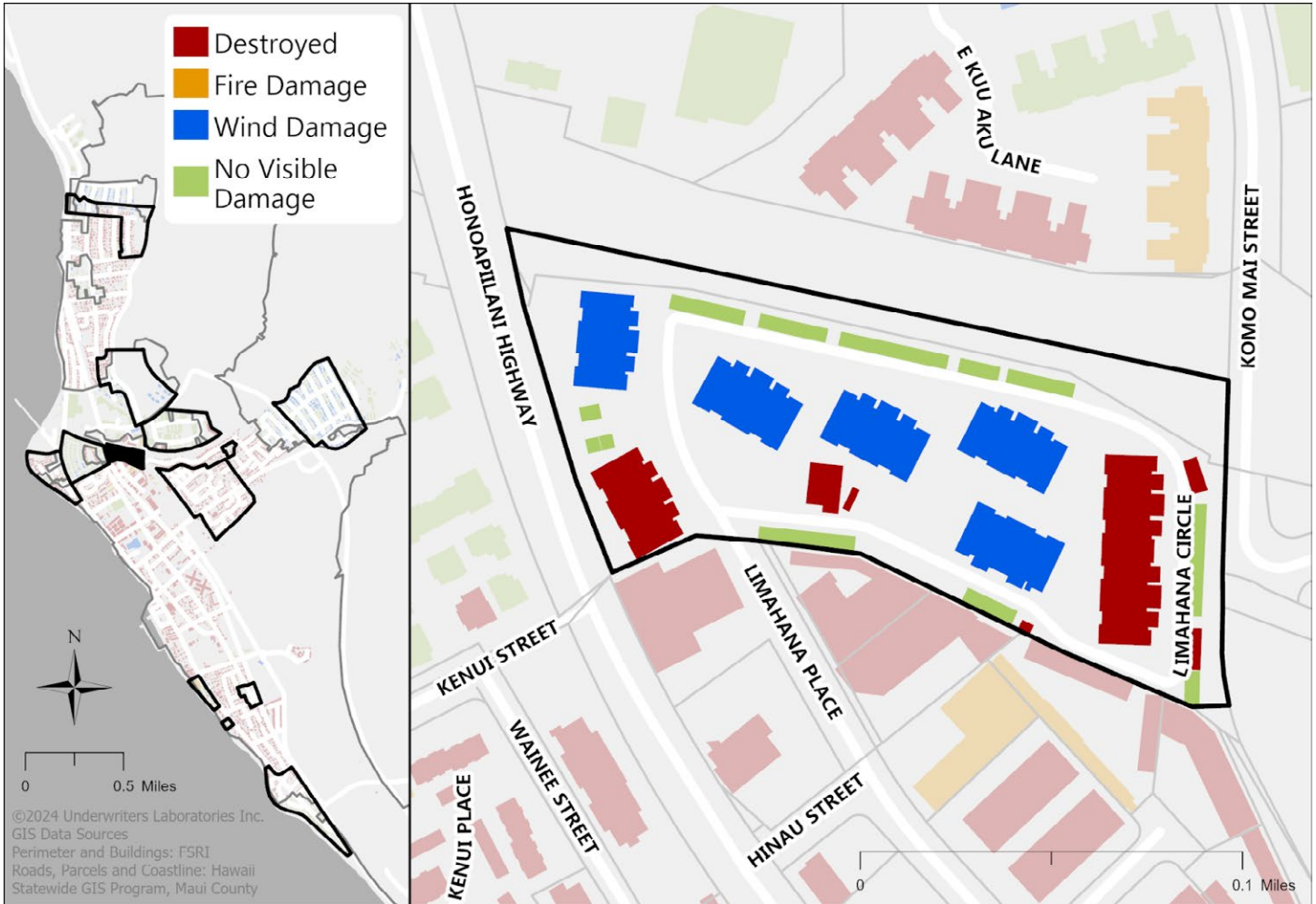
Figure 4.3.3.4.2 Damage classification assessment map of Opeukea apartment complex analysis area.
