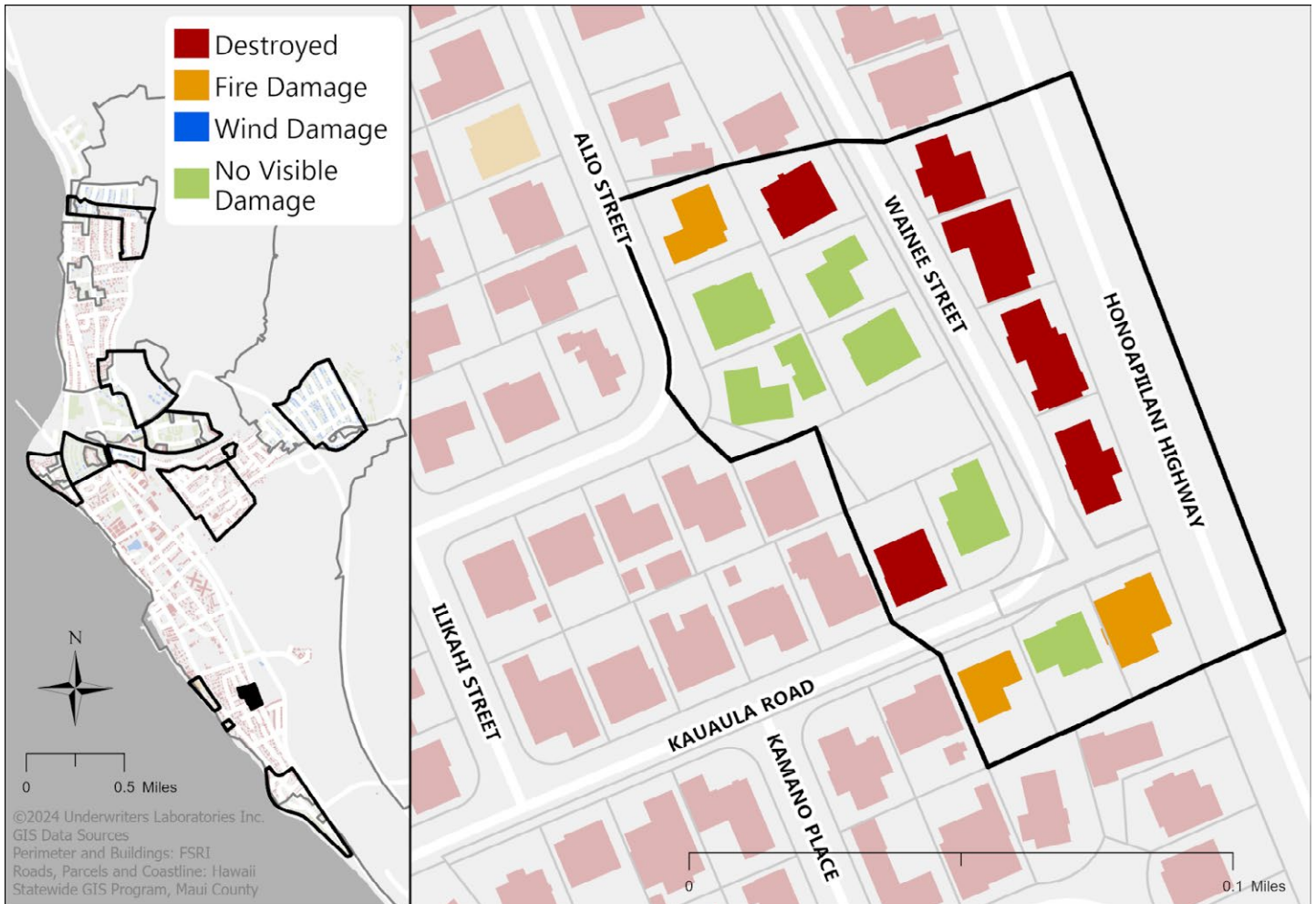
Figure 4.3.4.2.2 Damage classification assessment map of the 400 block of 'Ālī'ō and Waine'e Street analysis area.
