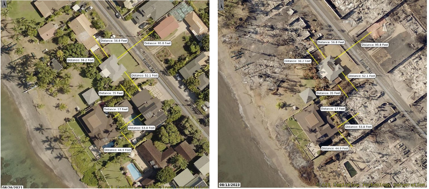
Figure 4.3.4.3.1 Surviving structures at 3 and 3 Front Street, including approximate separation distances determined from pre-fire images (left), which were superimposed on post-fire images (right).
