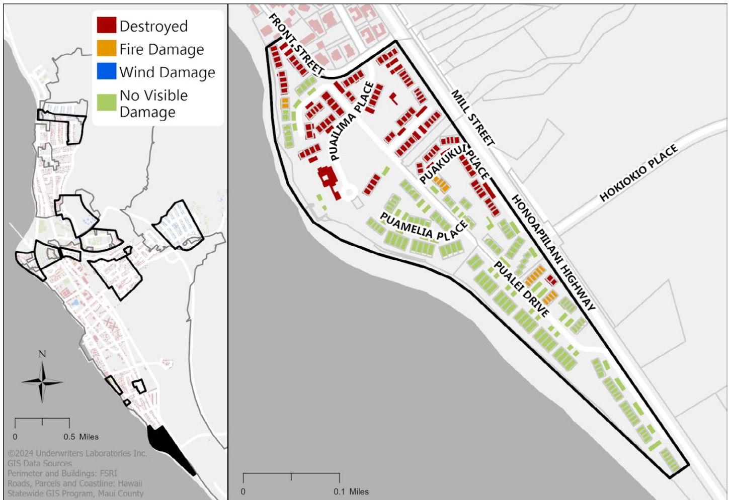
Figure 4.3.4.2 Damage classification assessment map of the Puamana Community analysis area.
