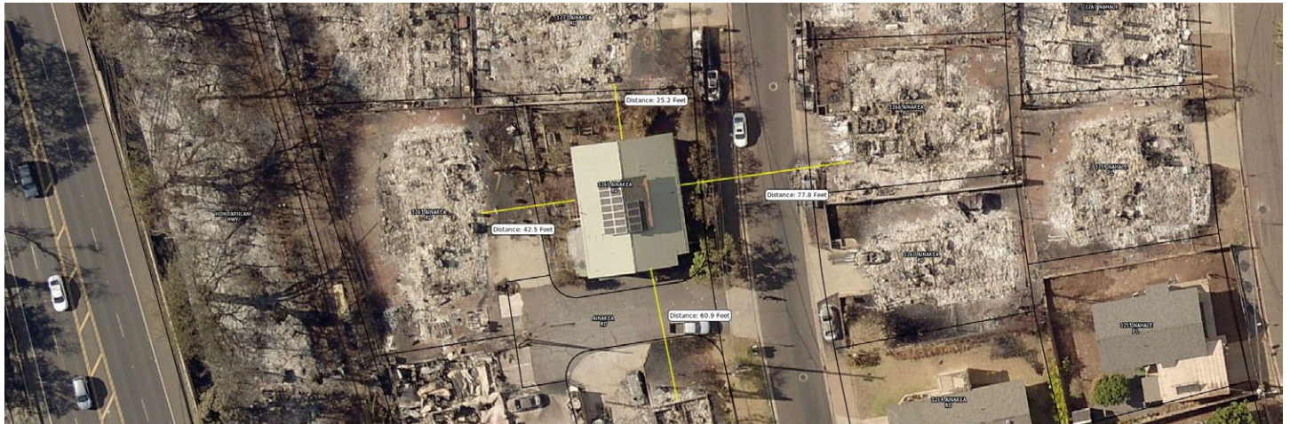
Figure 4.3.5.2.13 Post-fire aerial imagery of 12█ 'Ainakea Road with distances to adjacent (destroyed) buildings.
