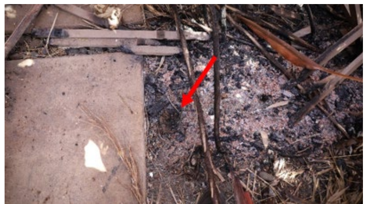
Figure 4.3.4.3.8 Gate and post moved away from burning fence pickets that interrupted the continuous wooden fuel from the 3█-3█ property line to the east (mauka) wall of 3█ Front Street. The charred end of the post remaining in the ground is indicated by the red arrow in the bottom right image.
