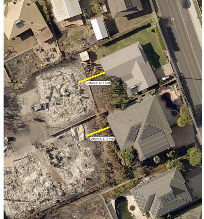
Figure 4.3.3.6.6 Destroyed structure on Lahilahi Place caused damage to the rear side of 11 (top) and 11 (bottom) Front Street structures.
