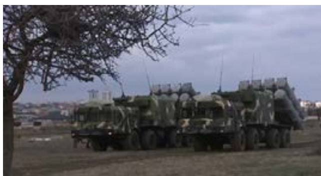
Surface-to-ship missile system "Bal" 【Official YouTube channel of the Russian Ministry of Defence】
