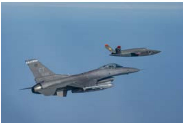
AI-controlled XQ-58A UAVs flying in formation with manned aircraft [U.S. Air Force]
