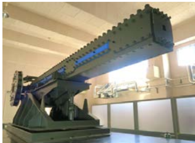
Railgun (electromagnetic gun) under research at the Acquisition, Technology & Logistics Agency (ATLA)
