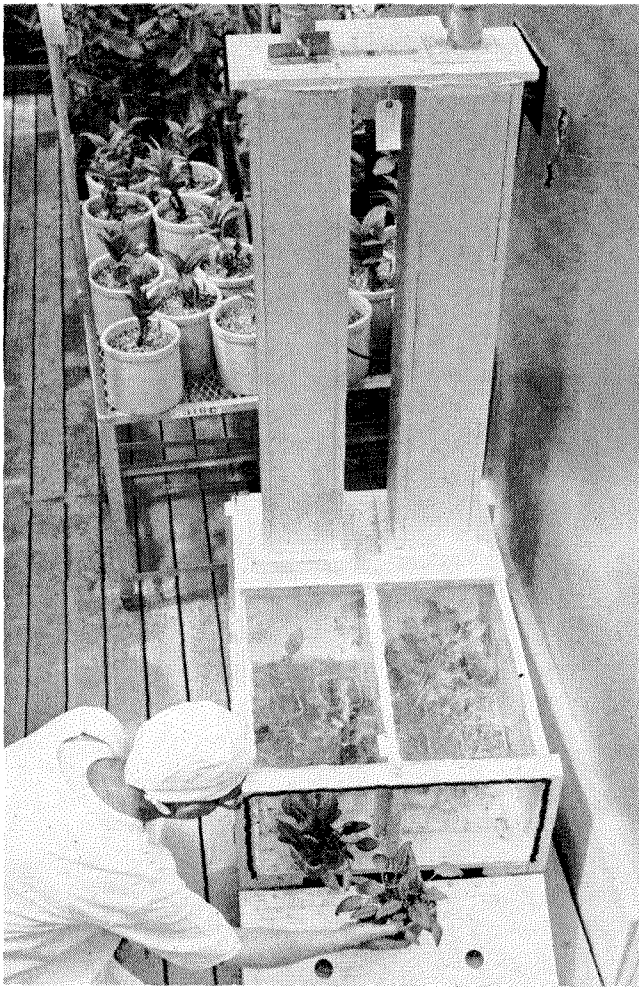
Smog damage to vegetables is studied at the Institute's Earhart Plant Research Laboratory. Smoggy air coming down the tunnel at the left, above, ruins plants. But the plants on the right keep healthy, since they're grown in air from which smog is removed by carbon filters.
