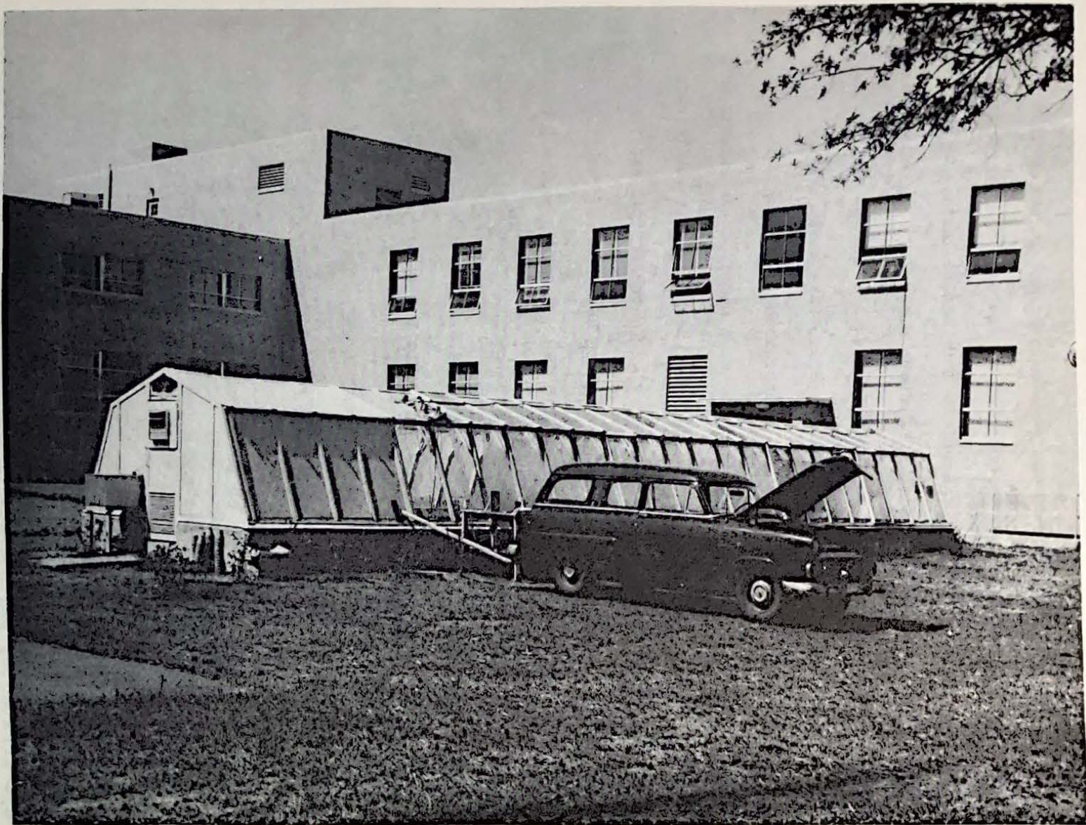
Chapter II - Fig. 4 Greenhouse Used for Experiments Irradiating Automobile Exhaust - Midwest Research Institute
