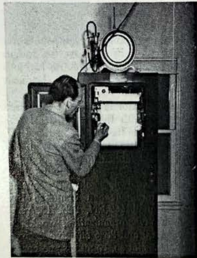
Sulfur dioxide content of atmosphere is continuously monitored by L. A. pollution control officials. Since inception of Air Pollution Control District, SO_2 content of air has been reduced 50%
