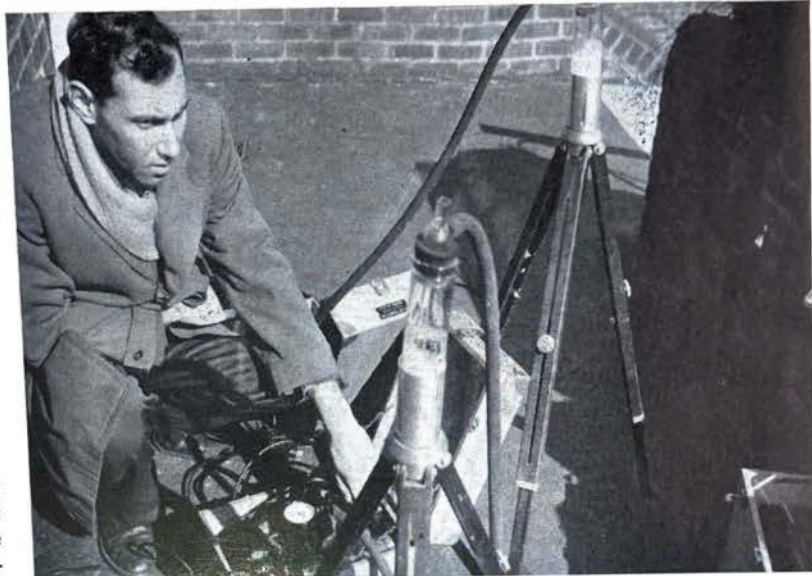
Employee of New York City Department of Air Pollution Control adjusts a Greenburg-Smith Impinger to check an odor complaint. Instrument checks amount of dust in the air and any specific gaseous pollutant which can be absorbed by use of various solutions in the tube. Complaint concerned electroplating plant, said to be venting fumes and annoying neighbors, who especially feared cyanide vapors. Tubes contained a 1% solution of sodium hydroxide
