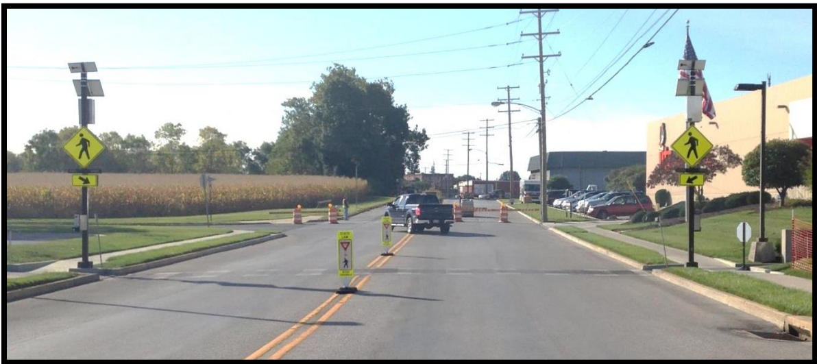
Figure 6: Example of "doubled up" Pedestrian Warning Signs with Rectangular Rapid Flashing Beacons
