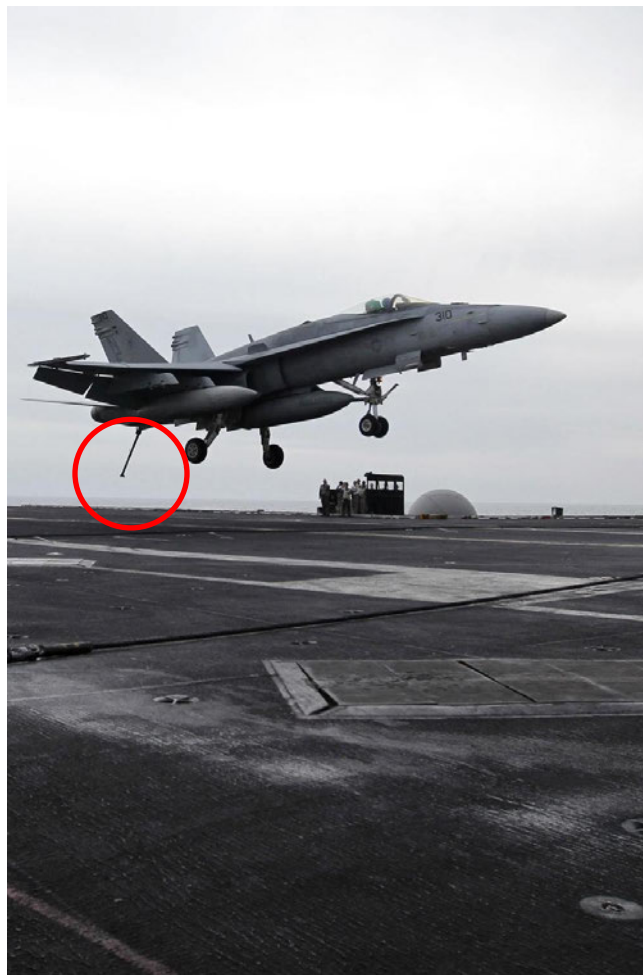
An FA-18 landing on an aircraft carrier at the correct angle. The tailhook (circled) and the two main mount wheels will hit the flight deck at the same time.
