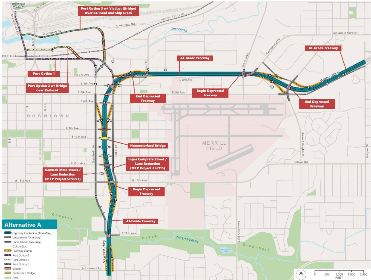
Figure 4. Alternative A: Roadway and Highway Improvements
