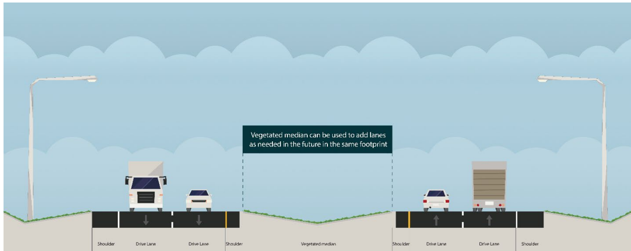
Figure 9. At-Grade Highway Cross Section (Six Lanes)
