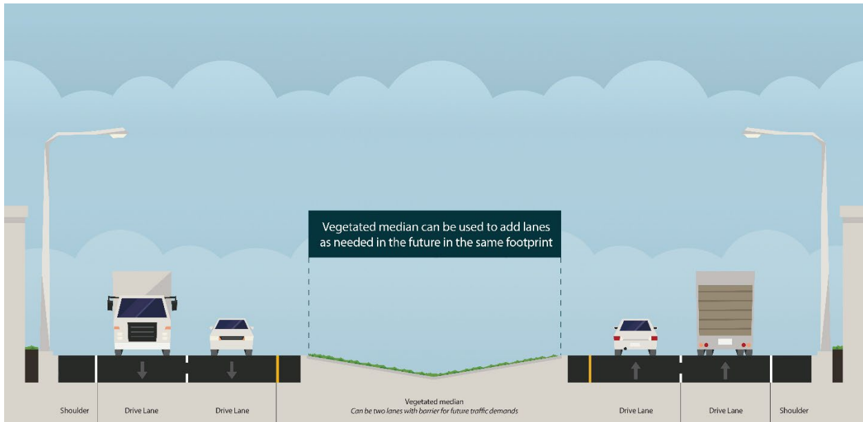
Figure 6. Depressed Highway Cross-Section (Four Lanes)
