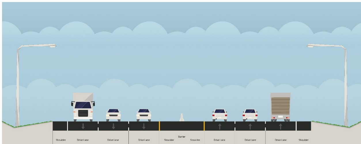
Figure 9. At-Grade Highway Cross Section (Six Lanes)
