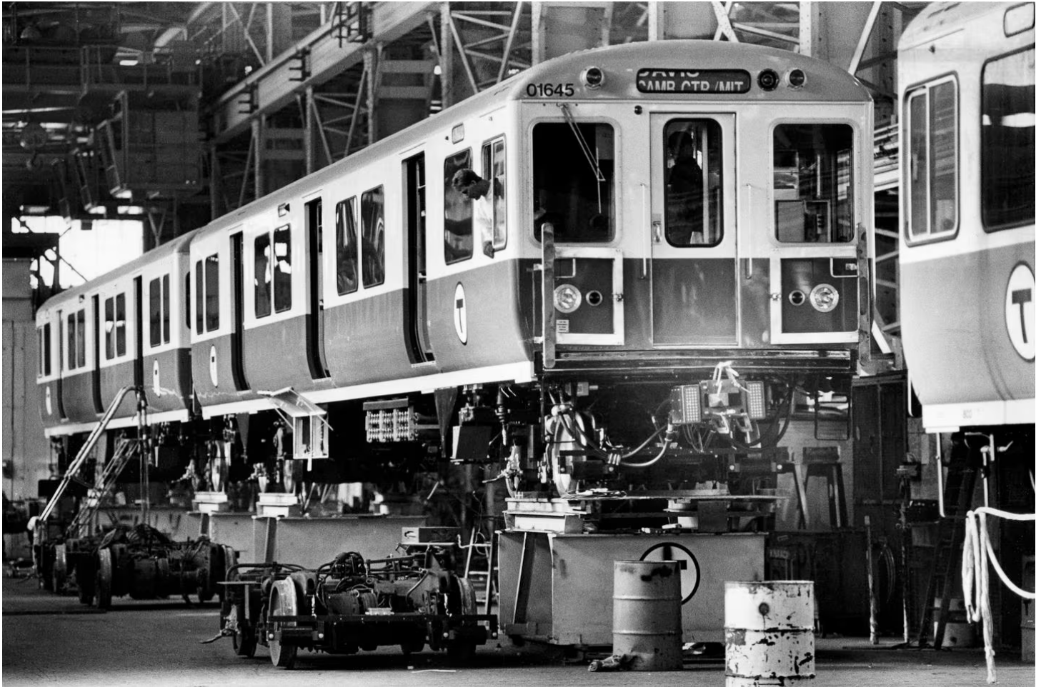
The Red Line “Silverbird” cars got a midlife rebuild in 1985. The project ran over six months late. The cars in the South Boston warehouse (pictured) were fitted with new parts in order for them to last another 10 years. DAVID L. RYAN/GLOBE STAFF
