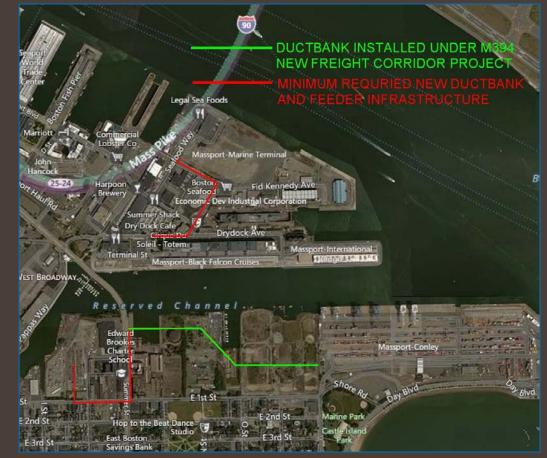
New Electrical Infrastructure to feed Shore-to-Ship Power at Conley Terminal From Eversource K Street Substation
