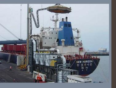
Covers the stack of a vessel, vacuums the exhaust of the vessel, and treats the exhaust.
