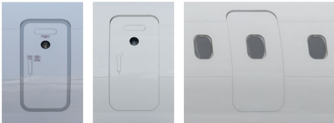
Figure 2. Diagram showing the mid exit door locations. (Source: Boeing. Image Copyright © Boeing. Reproduced with permission.)
