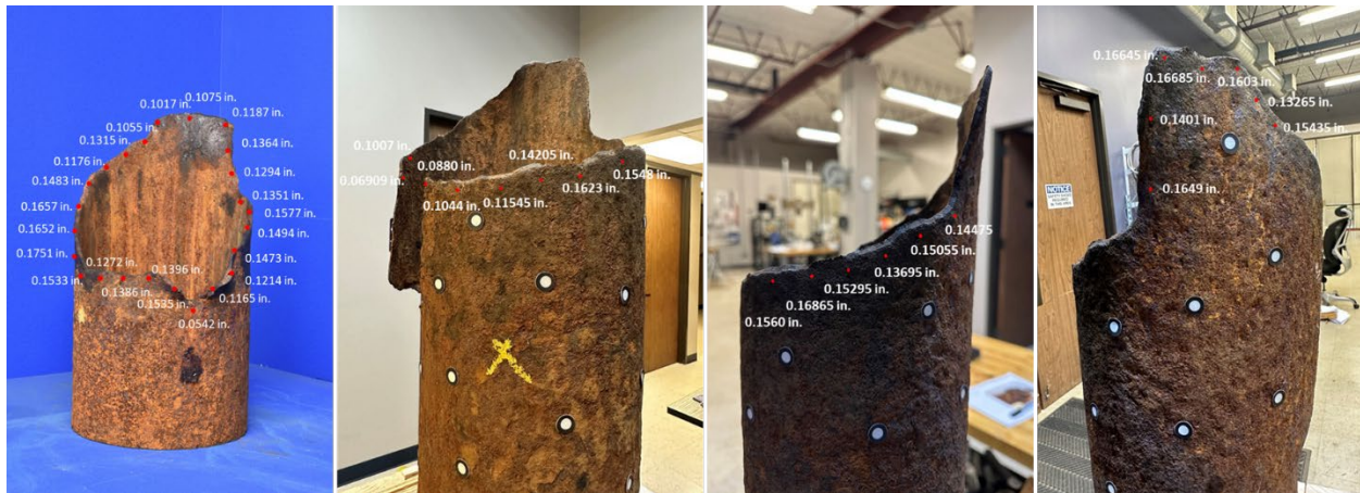
Figure 70: Thickness Measurements along the Circumferential Fracture Surface of C001B-1 and C001A
