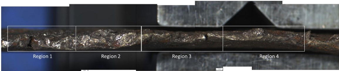
Figure 58: Different C001A-2A Regions Examined in the SEM
