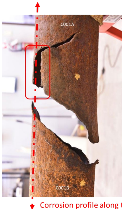
Figure 88: Orientation of Thickness Profile Used for Burst Pressure Estimation
