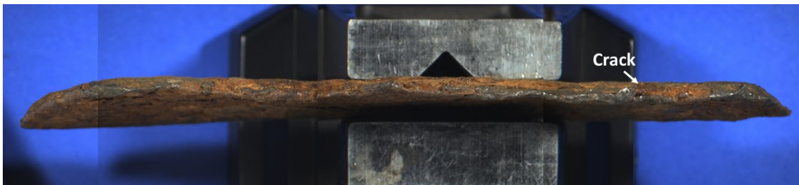
Figure 35: Stitched Stereoscope Image of C001A-1 Fracture Surface
