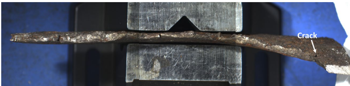
Figure 36: Stitched Stereoscope Image of C001A-2 Fracture Surface
