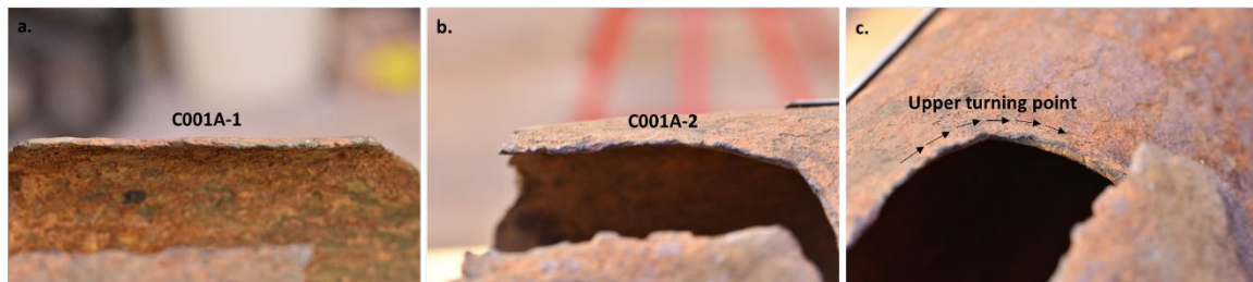
Figure 30: Axial Rupture Fracture Surfaces (a) C001A-1, (b) C001A-2, and (c) Upper Turning Point
