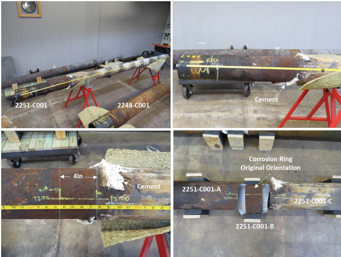
Figure 113: C001 Joint from Well #2251 Before and After Cutting
