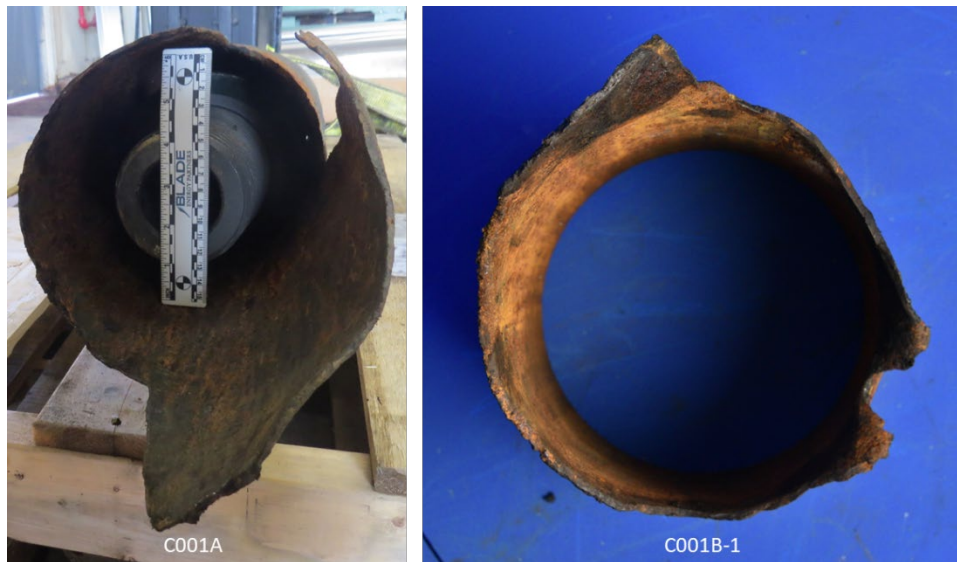
Figure 71: Circumferential Fracture Surfaces from C001A and C001B-1
