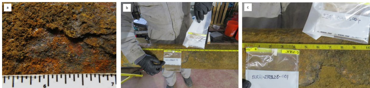
Figure 118: Example of OD Surface Scale and Deposit Collection and Bagging
