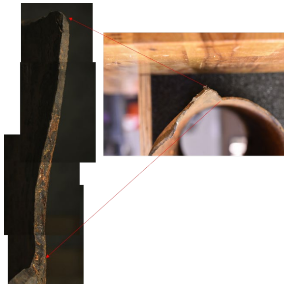
Figure 74: Stitched Stereoscope Image of the Step in Circumferential Fracture Surface in C001A
