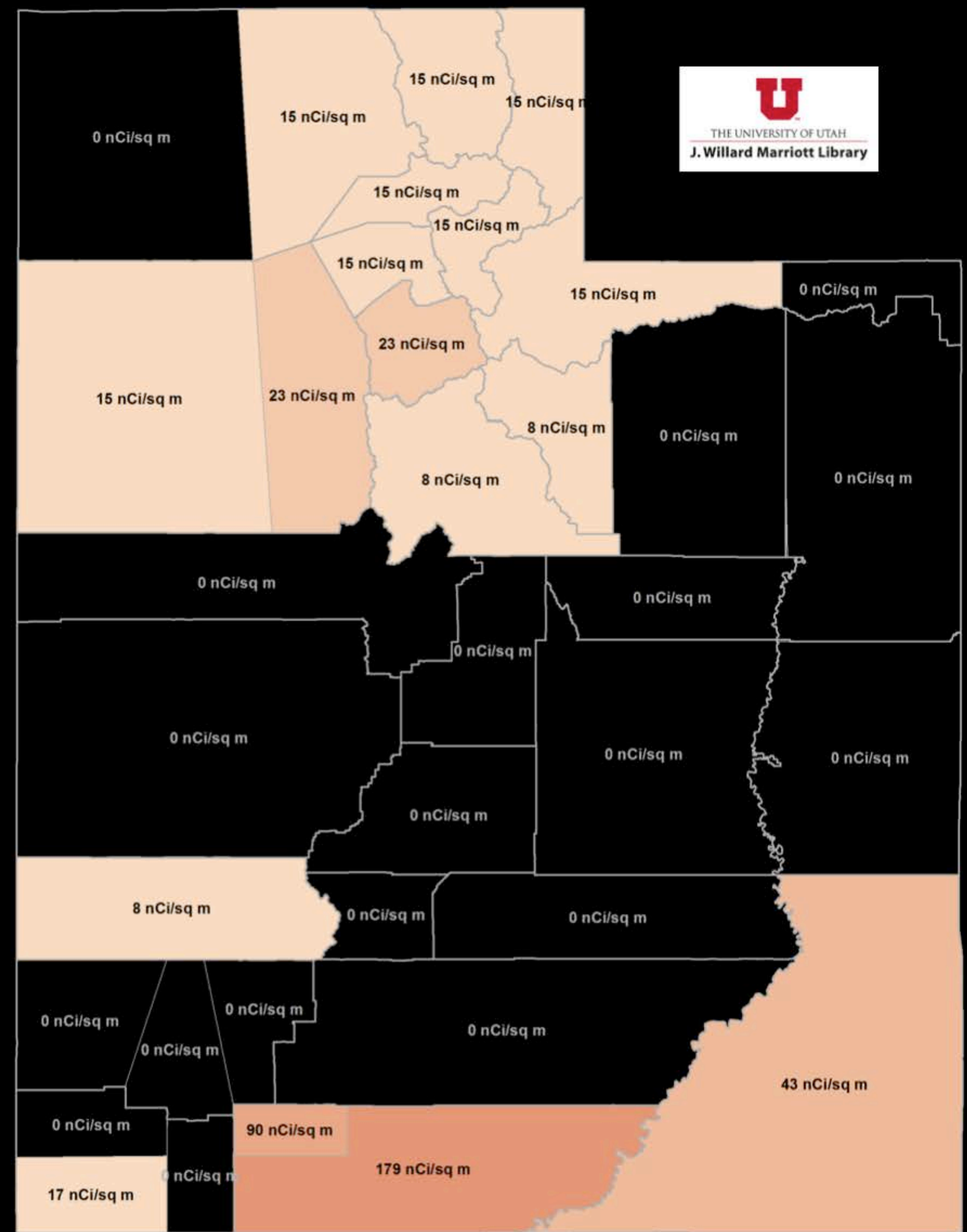
Data figures were produced as part of the National Cancer Institute study: Estimated Exposures and Thyroid Doses to the American People from Iodine-131 in Fallout from Nevada Atmospheric Nuclear Bomb Tests. These figures represent the geometric mean for the average ground depositions (nCi/sq. m) for each county within Utah related to this event.
