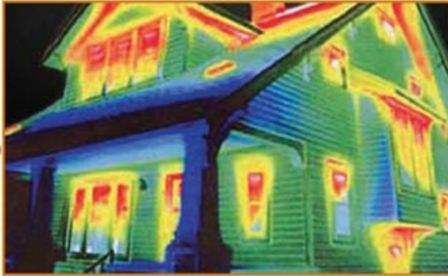
Figure 10: Most household heat loss is through the windows and roof. Source, U.S. Department of Energy.
