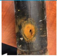
**Artifact 1:** A small pinhole in the fire sprinkler pipe caused a flood in the Andrew Robinson media center
