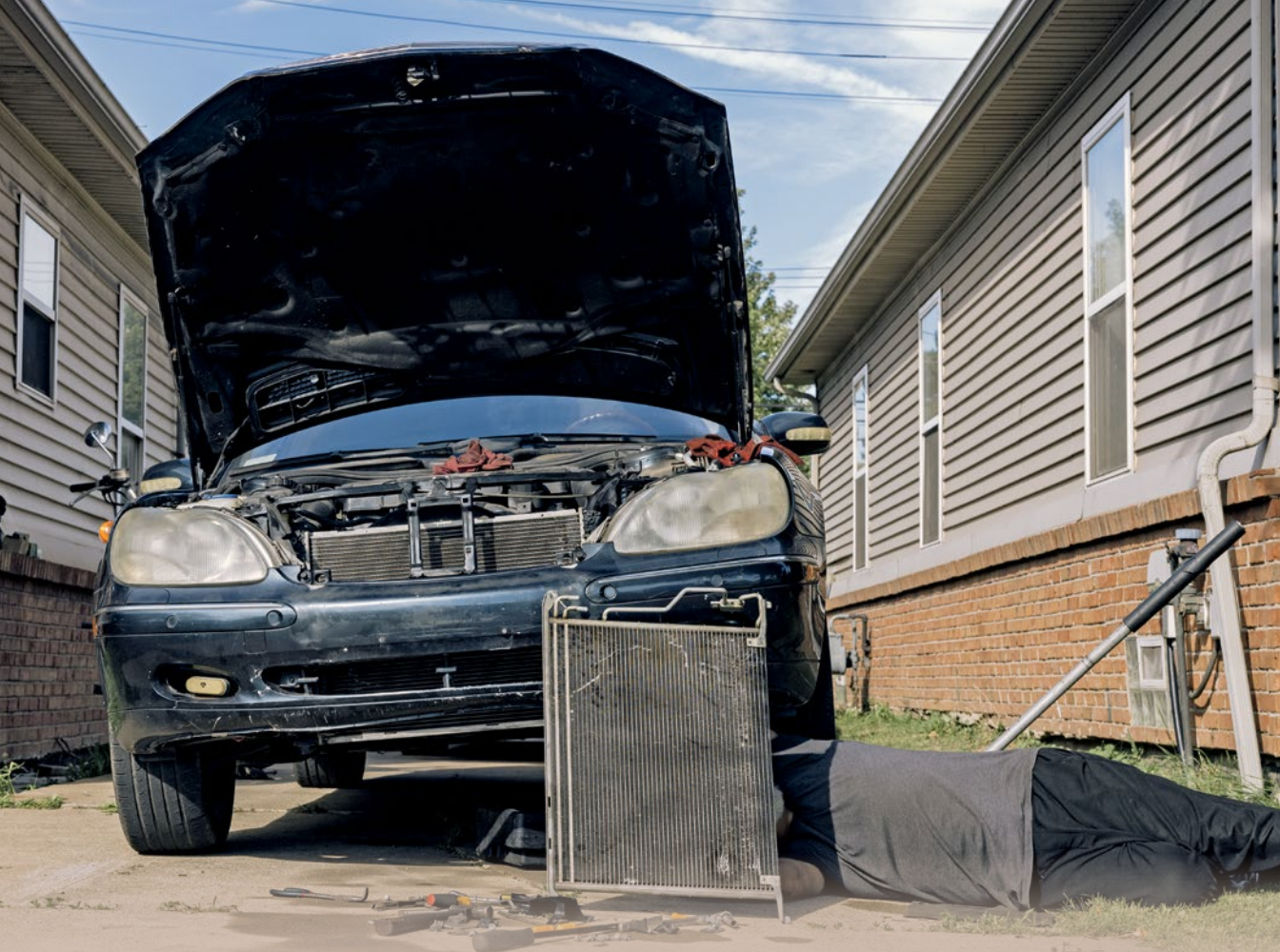
Fixing a broken AC condenser on a used car in Dearborn, Michigan.
