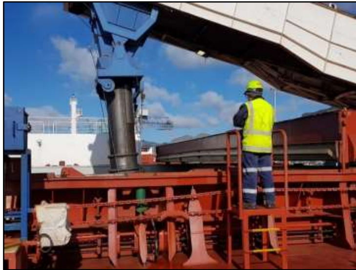
Figure 20: Photo in SWMS showing the signalman standing on a pedestal looking over the hatch coaming into the hold
