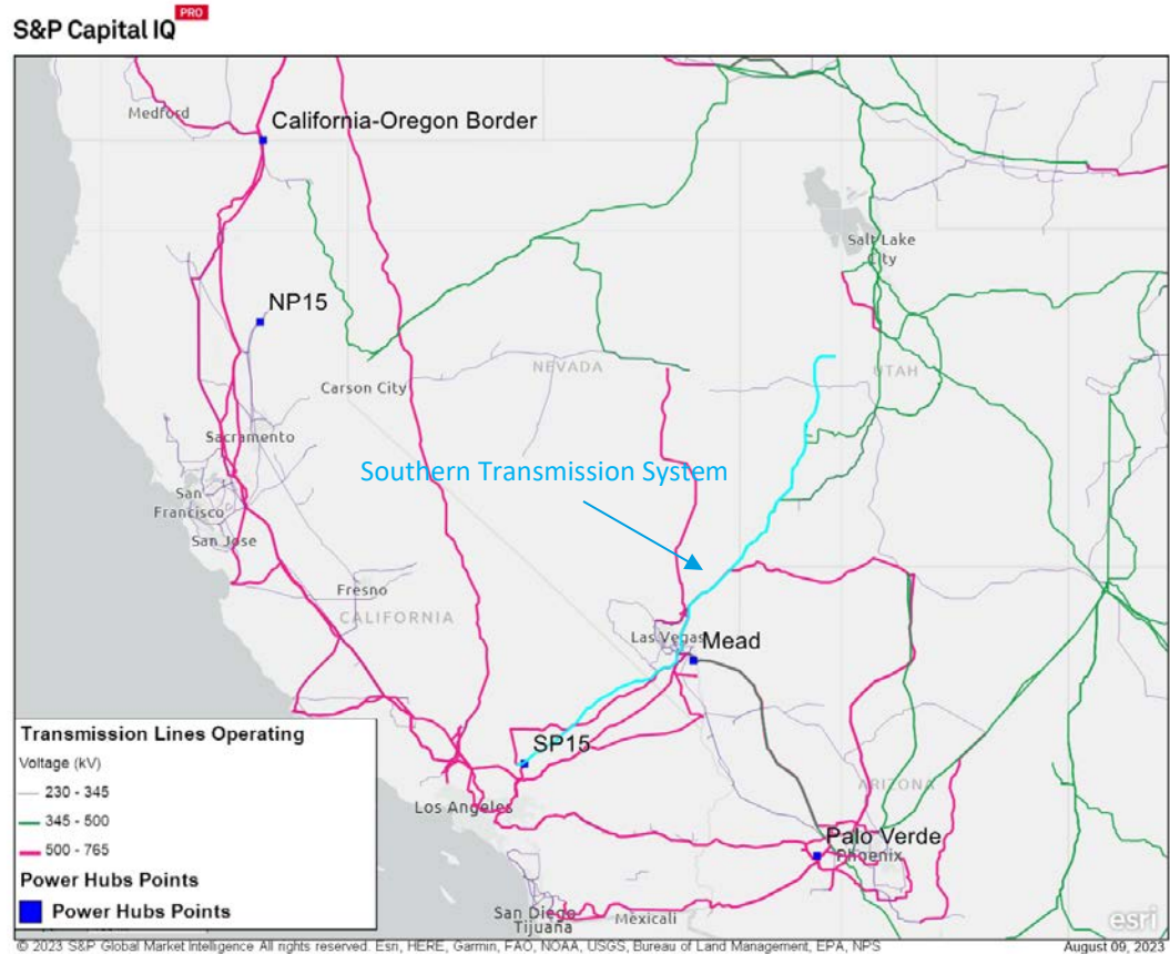
Figure 2. High voltage (230kV+) transmission lines and power wholesale market hubs in the southwest
