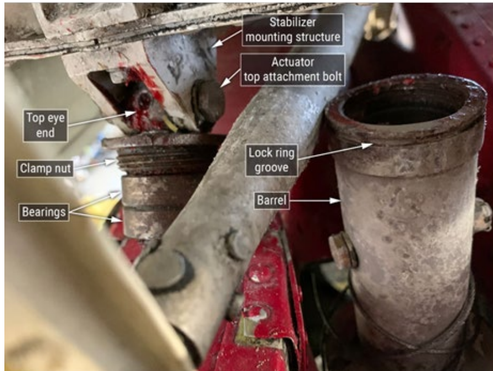
Figure 7. Photograph of the clamp nut and barrel separation on the accident airplane.
