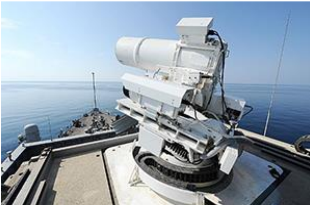
Figure 2. Laser Weapon System (LaWS) on USS Ponce
