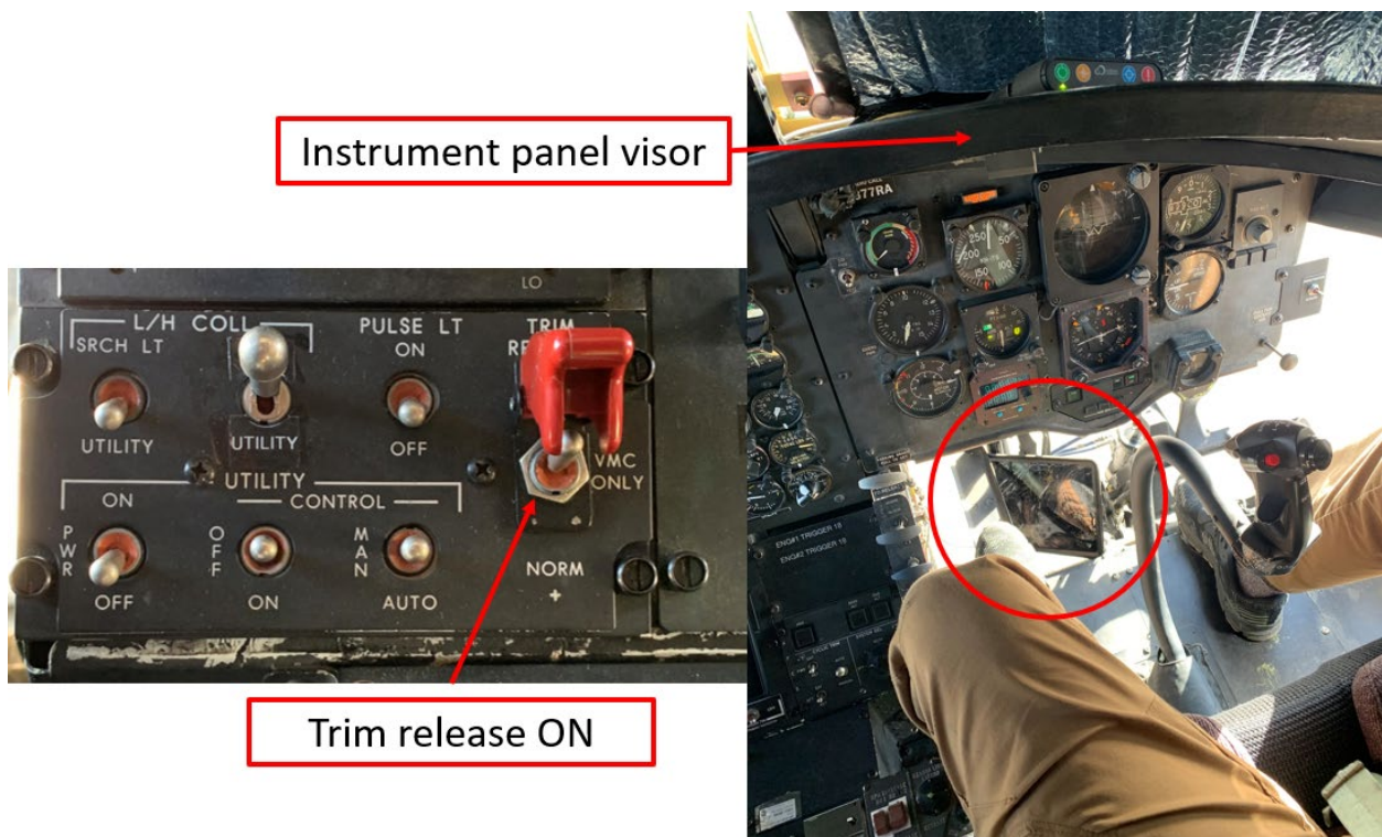
Figure 2. Trim release ON and iPad placed in co-pilot's left pedal area.
