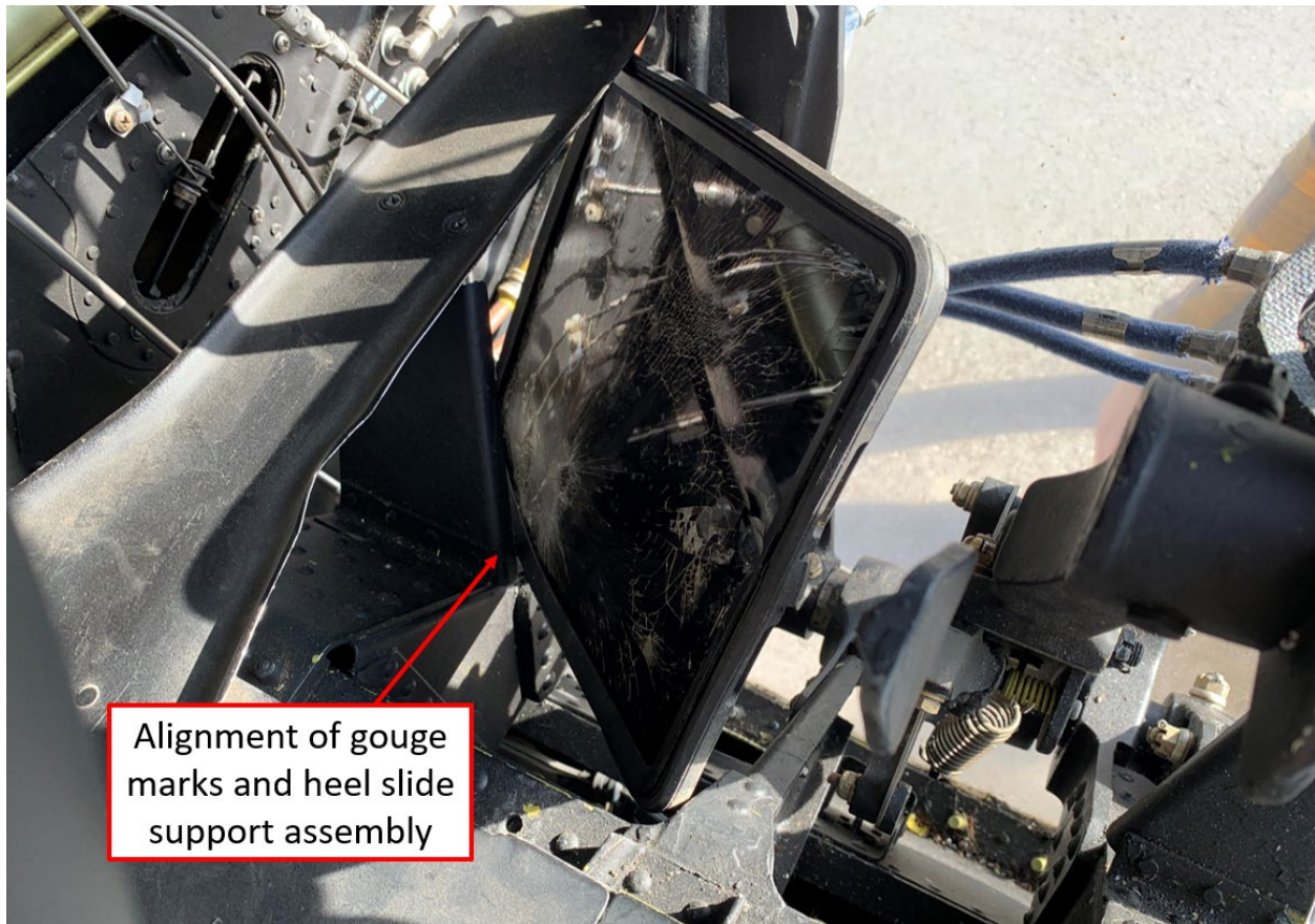
Figure 5. The iPad impinged in between the co-pilot's left pedal and the airframe. The lower left corner of the iPad is lodged into a small corner of the airframe. The gouges in the iPad aligned with a sharp, vertical metal piece of the heel slide support assembly.
