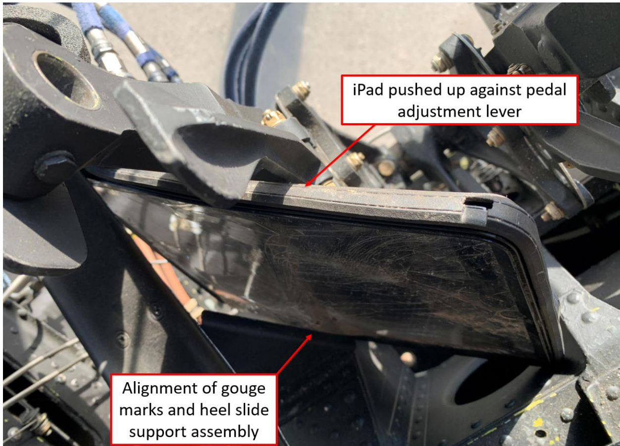
Figure 4. The iPad impinged in between the co-pilot's left pedal and the airframe. The back side of the iPad is pushing against the left pedal adjustment lever. The lower left corner of the iPad is lodged into a small corner of the airframe. The gouges in the iPad aligned with a sharp, vertical metal piece of the heel slide support assembly.
