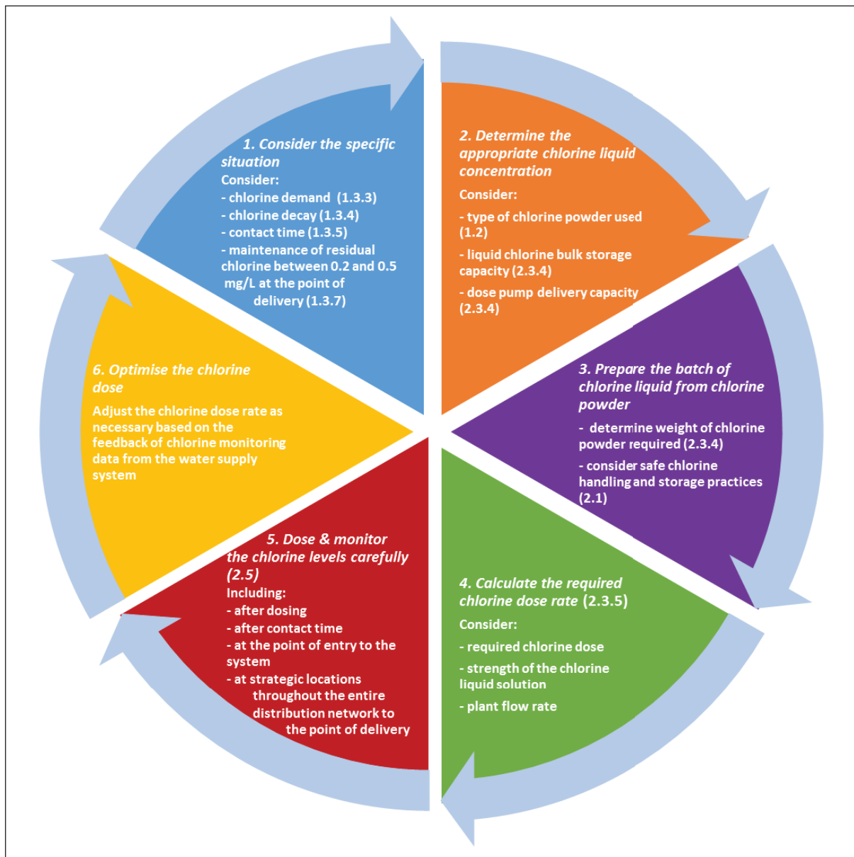
Figure 15. Key steps for effective chlorine disinfection of drinking-water using chlorine powder 30 (section references are presented in parentheses)
