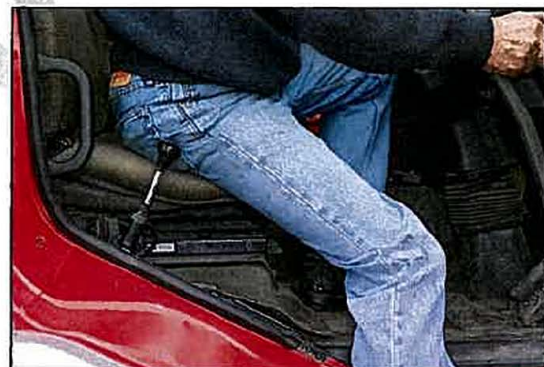
Figure 7 – Contact with the park brake when exiting the truck [60000]
