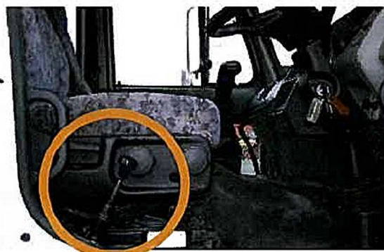
Figure 2: shows the interior of a truck cab with a park brake control valve positioned at the base of the driver's seat. The park brake is in the "engaged" position.
