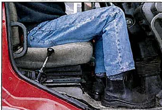
Figure 6 – Location of engaged park brake with driver seated [60000]
