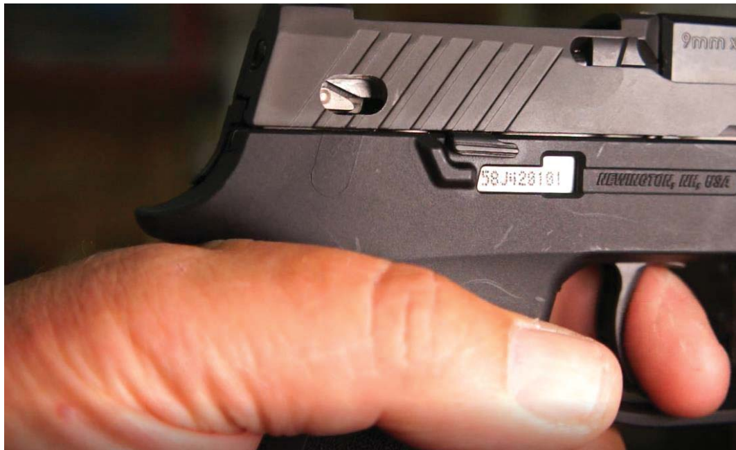
The firing pin block disengaging with less than .075” of a trigger pull under less than 1.5 pounds of pressure on an exemplar P320. See Appendix E.
