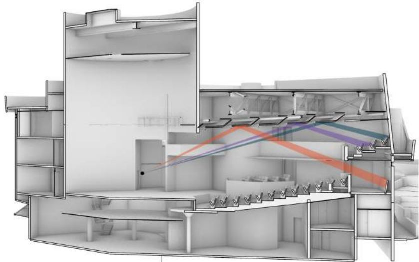
Acoustics Figure 23 Current Balcony and Audio Mix Ceiling Reflections - Midstage Source
