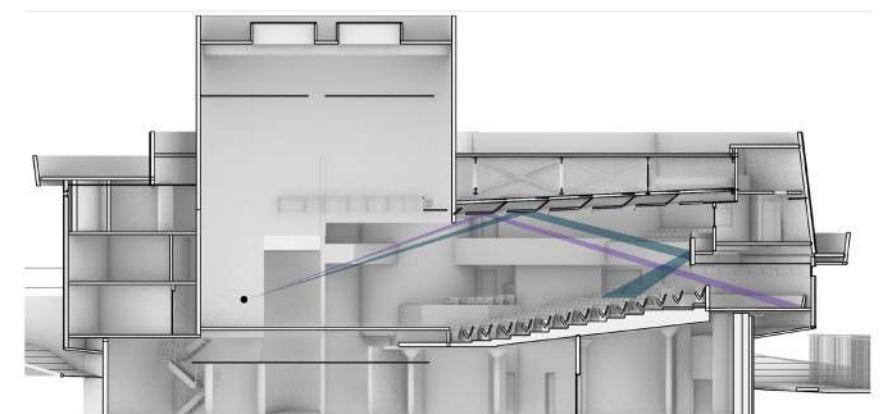
Acoustics Figure 18 Current Audience Ceiling Reflections - Upstage Source
